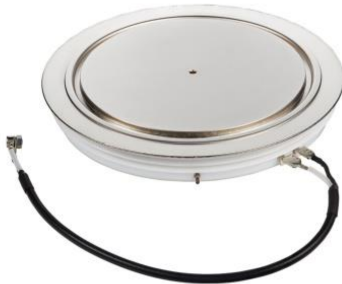
Figure. Infineon's Press Pack IGBT features a blocking voltage of 4.5 kV at 3000 A without FWD and 2000 A with FWD. Fitting to the 3000-A device, Infineon offers external freewheeling diodes in different silicon diameters. According to the vendor, leading high-voltage IGBT chip trench technology combined with highly reliable press-pack technology, proven in the field for more than 40 years, provides customers with an excellent, high-performance solution for ultra-high power applications. In addition, the devices open up new opportunities to optimize high-power applications in terms of losses, reliability and cost.
