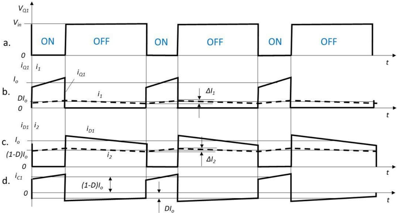
Fig. 4. Voltage and current waveforms in the continuous-input current regulator shown in Fig. 2. Input current ( $i_1$ ) waveform (dashed line in diagram b.) is distinctly different from the conventional case and represents a continuous function of time.
