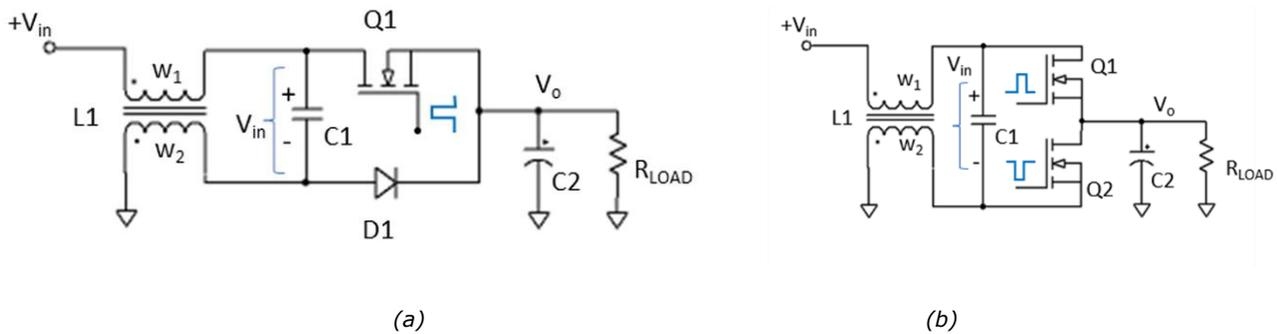
Fig. 2. Enhanced buck converter topology with continuous input current (a). The current of each inductor winding can pass through the cap and sequentially flow either through closed switch Q1 or conducting diode D1. The same topology can also be implemented with a synchronous FET in place of the freewheeling diode (b).
