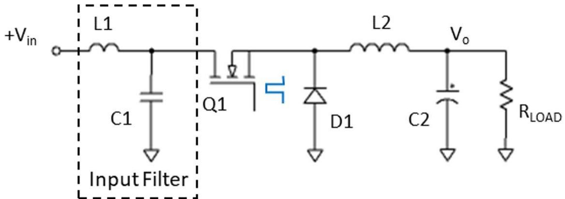
Fig. 1. Basic stepdown voltage regulator. Input LC filter components reduce voltage spikes on Q1 and D1 and smooth the current drawn by the converter to keep the host supply voltage within the required range.
