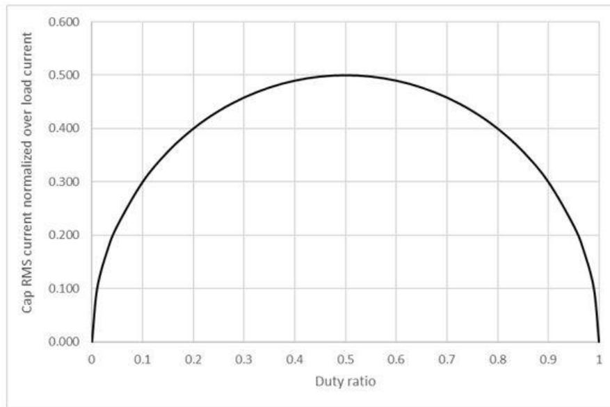
Fig. 6. Normalized input cap RMS current vs. duty ratio.
