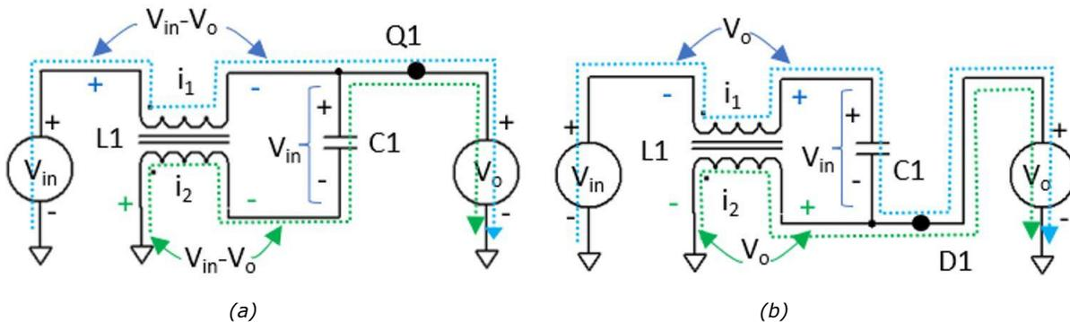
Fig. 3. Continuous input current VR equivalent schematics for switch-on (a) and switch-off (b) time intervals.
