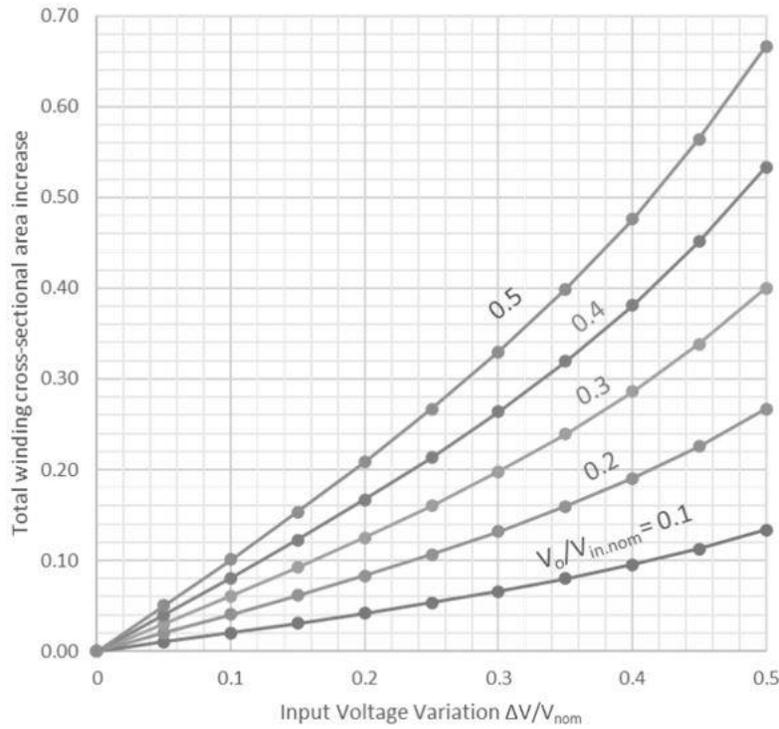
Fig. 5 Inductor winding cross-sectional area increase (k) in the modified VR vs. input voltage variation and output-to-input voltage ratio.
