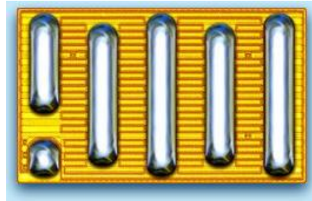
Fig. 1. The first of EPC's Gen 6 devices, the 80-V, 4-mΩ EPC2619 GaN FET in a 1.5-mm x 2.5-mm footprint offers higher performance than the company's Gen 5 devices and further widens the performance advantage of the company's GaN FETs versus traditional silicon MOSFETs. The improvements benefit high power density applications, including dc-dc conversion, motor drives, and synchronous rectification.
