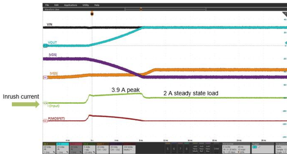
Fig. 8. R5 SOA performance in the TO-257AA package limits use to <50-W converters in inrush current limiting applications.
