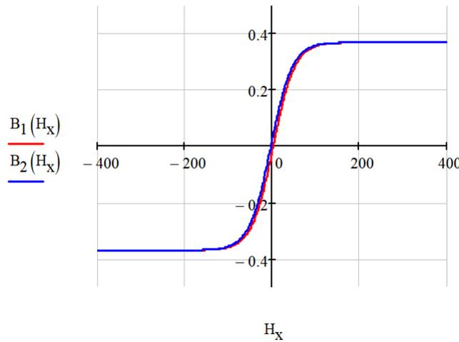
Figure. Hysteresis loop model for a real core (an R34 toroid core made of N88 ferrite material.)
