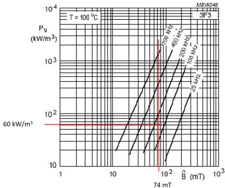
Fig. 4. Specific power loss as a function of peak flux density with frequency as a parameter (courtesy of Ferroxcube).
