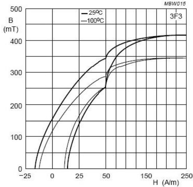
Fig. 3. BH curves (courtesy of Ferroxcube).
