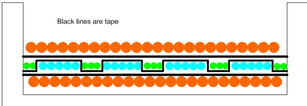
Fig. 6. Coupled inductor layout.
