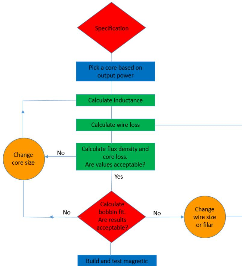
Fig. 1. Design flow for a coupled inductor.
