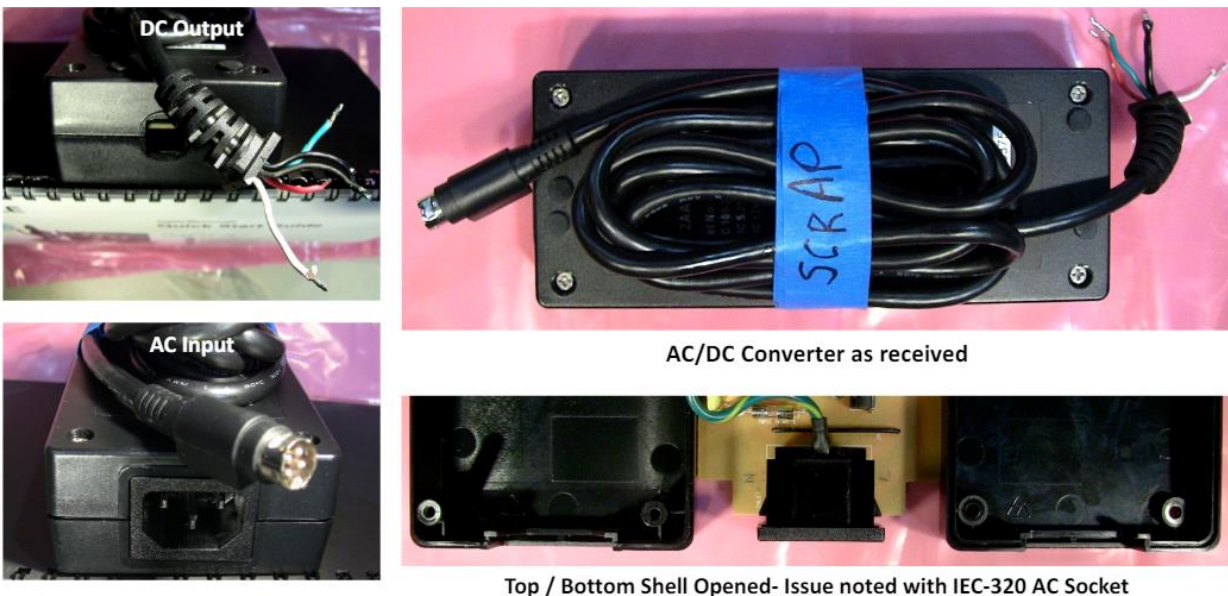
Fig. 8. This ac-dc power supply with a switchable (120 or 240 V) input failed after undergoing vibration qualification tests. When the unit was partially disassembled by the customer as shown here, an issue with the ac socket was discovered. (Courtesy of Collins Aerospace and CMSE 2024.)
