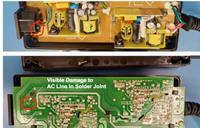
Fig. 9. Inspection of the power supply's pc board revealed a failed solder joint on the ac connection to the board was responsible for the power supply failure. But was the failure caused by the vibration testing? (Courtesy of Collins Aerospace and CMSE 2024.)
