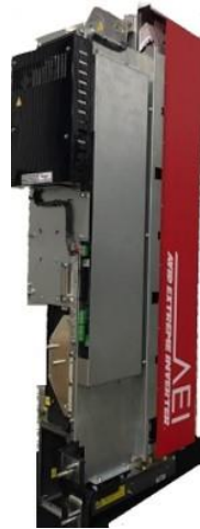
Fig. 1. The Avid Extreme Inverter modules are high-reliability liquid- and air-cooled inverter modules with nominal ratings from 550 A to 1400 A and up to 690 Vac for use with MV3000 AC drives, controlled by the Common Drive Controller (CDC).
