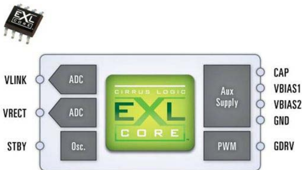
Fig .1 The CS1500 and CS1600 PFC controllers are based on the company's EXL Core architecture, a digital technology platform.
