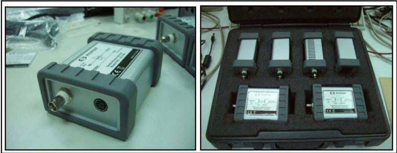
Figure. With its 10-Hz to 45-MHz bandwidth, the J2101A injection transformer can support control loop stability analysis for designs ranging from offline power supplies to state-of-the art, multi-megahertz switching regulators. Another model, the J2100A features a bandwidth that extends down to 1 Hz. The 0- to 50-MHz solid-state signal injector is pictured above (photo on left) with the Injector Bundle Kit (photo on right).
