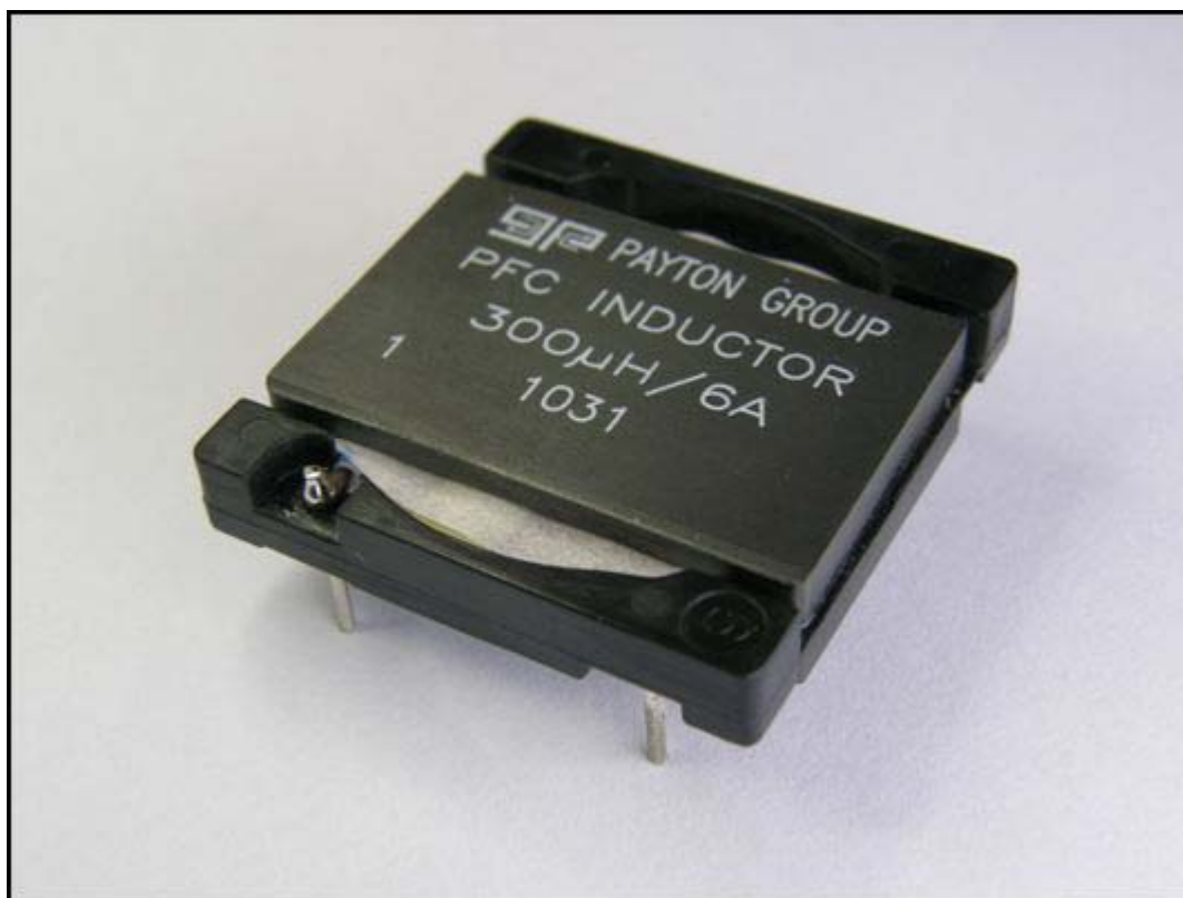
Figure. This 8-mm high planar inductor enables the development of 200-W power supplies with a profile of less than 1 cm as required in large-format LED televisions.
