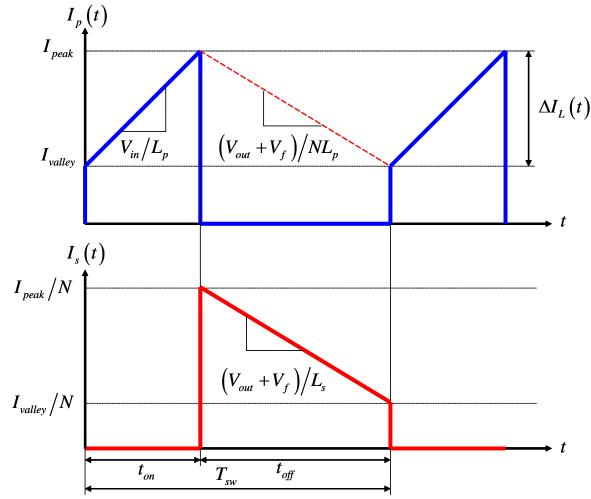
Fig 2. In CCM, the current first ramps up in the primary side until the switch opens and transfers the stored energy to the secondary side.
