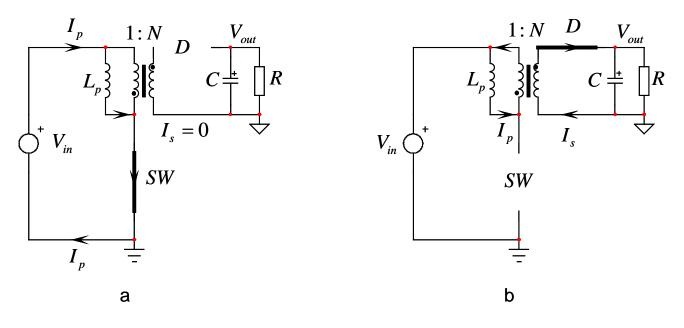
Fig.1. The two operating states of a flyback converter show energy storage in the primary side (a) followed by energy circulation in the secondary side (b).
