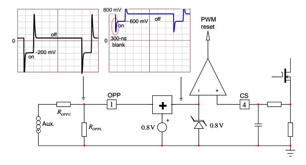
Fig. 9. Sensing the auxiliary winding of the flyback converter during the on time is an excellent way to obtain an image of the input voltage without incurring additional power dissipation.
