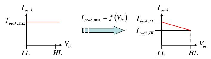
Fig. 6. One approach to implementing over-power protection is to limit the peak current as a function of input voltage.
