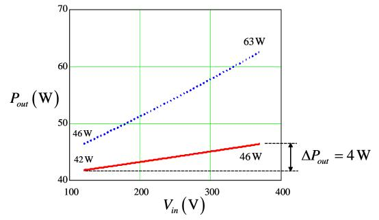
Fig. 10. OPP implementation clearly improves the output-power limiting of the flyback converter.
