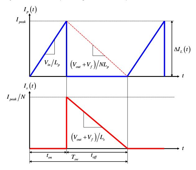
Fig. 3. When the flyback converter operates in DCM, the inductor current ramps up from zero.
