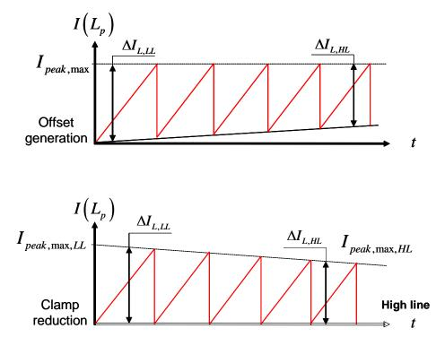
*Fig. 7. The reduction in the peak-current limit at high line can be obtained by either offsetting the current-sense signal (top graph) or by reducing the internal clamping value (bottom graph).*
