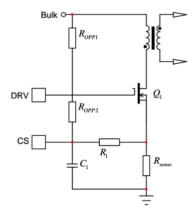
*Fig. 8. By generating an offset from the bulk capacitor to the current sense pin, we can create a variable offset affecting the maximum output power of the converter.*
