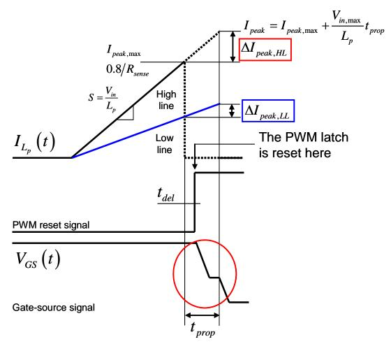
Fig. 5. When an overcurrent condition is detected, it takes a certain amount of time before the controller acknowledges the fault and propagates the turn-off signal to the MOSFET gate.
