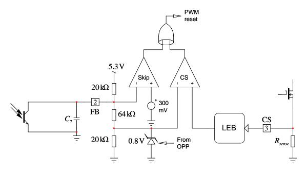
*Fig. 4. The maximum peak current is set by the 0.8-V reference voltage.*
