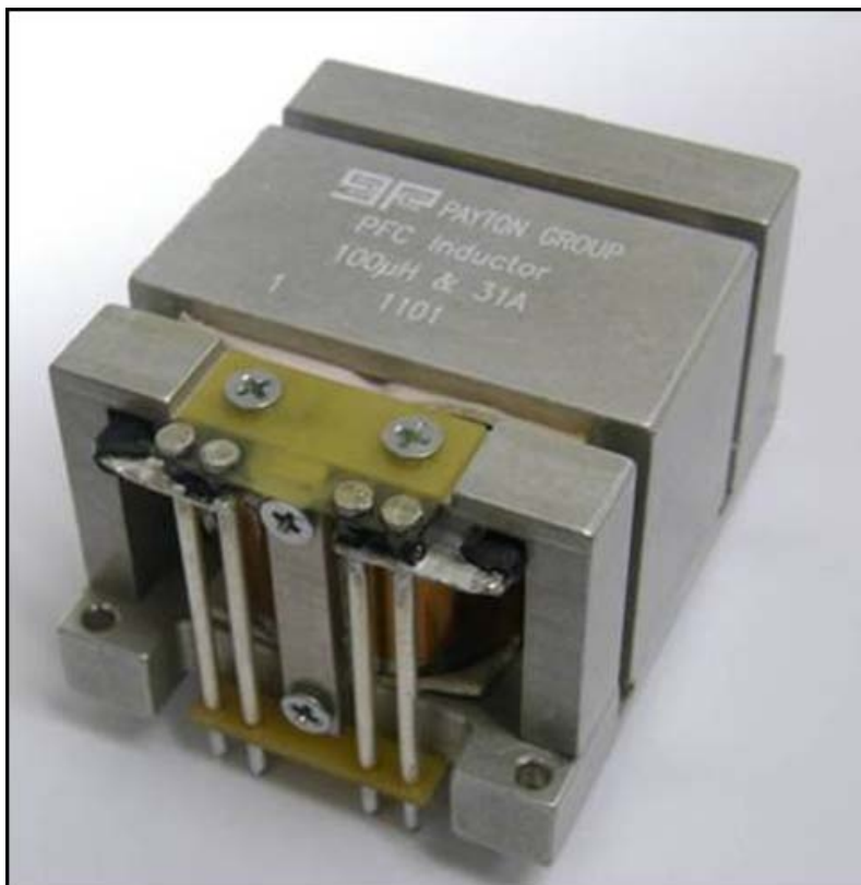
Fig. Payton Planar Magnetics' new line of PFC boost inductors employ Metglass (amorphous) or nanocrystalline core material to achieve high-power, compact designs. This example inductor, which measures 70 mm (L) x 55 mm (W) x 40 mm (H), is designed for a 5000-W system. The core is a special design produced using nanocrystalline material.
