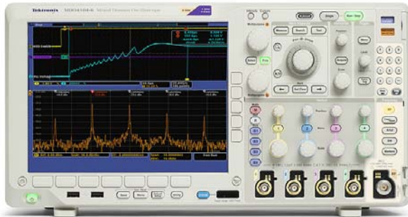
Tektronix MDO4000 series oscilloscope with built-in spectrum analyzer.
