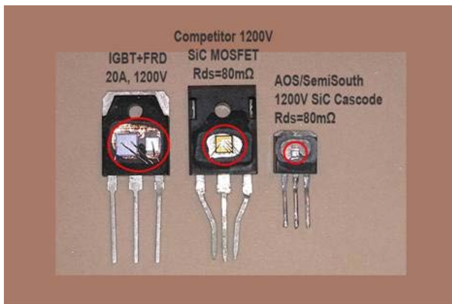
Figure. Comparison of die sizes for the UniSiC Stack-Cascode MOSFET from Alpha and Omega, a SiC MOSFET, and an IGBT with co-packaged fast recovery diode.
