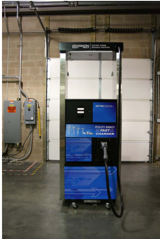
Fig. 2. As proof of concept for EPRI's Utility Direct Fast Charger technology, EPRI's developed and demonstrated this prototype of a 2.4-kV 45-kVA solid-state, dc fast charging system for electric vehicles.
