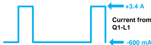
Fig. 11. Total current supplied by Q1 and L1 of the SEPIC-coupled quadrupler in Fig. 9.
