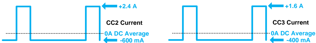
Fig. 11. Waveform for current through CC2 and CC3 of the SEPIC-coupled quadrupler in Fig. 9.
