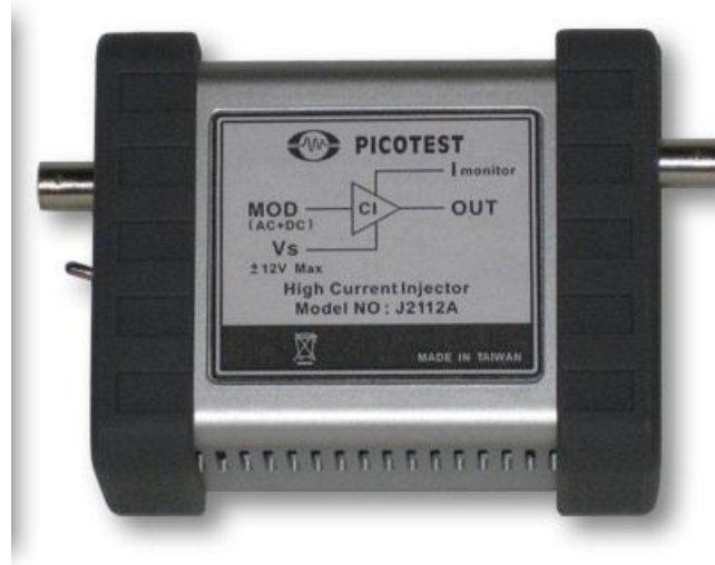
Fig. 1. Picotest's J2112A fast current injector is a higher-current version of the company's popular J2111A. When compared with that current injector, the new J2112A offers a greater current range (1 A vs. 100 mA) while improving rise/fall times down to 10 ns and achieving greater than 40-MHz bandwidth.
