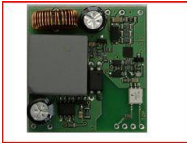
Fig. 2. This discrete SiC BJT driver board from Fairchild Semiconductor is a plug-and-play solution.
