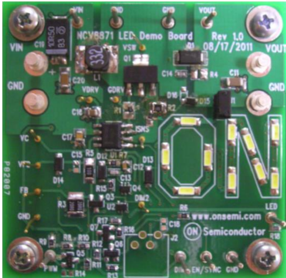
Fig. 2. Demonstration board for the dimmable LED driver circuit shown in Fig. 1.
