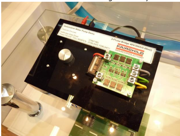
Fairchild Semiconductor's FTCO3V455A1 three-phase, variable-speed-drive automotive power module.
