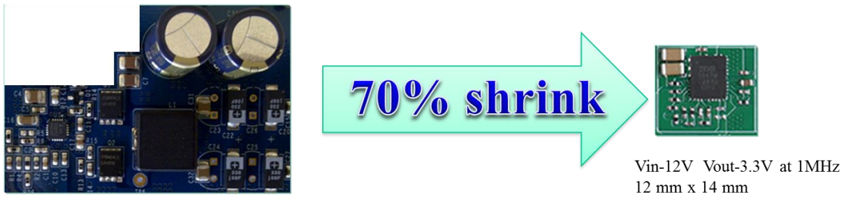
Fig. 5. With its 1-MHz switching frequency, the IR3847 shrinks the PCB footprint required for a 25-A point-of-load converter so that it can be implemented in as little as 168 mm 2 of board space.
