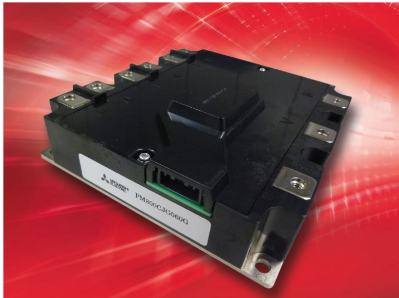
Fig. To meet stringent EV and HEV demands for safety and reliability, while also satisfying requirements for higher current handling ability, Mitsubishi Electric has added two new members to its J series of intelligent power modules. Implementing a 3-phase inverter configuration, the new IPMs use low-loss CSTBT chip technology to provide ratings of 600 V and 800 A with a low saturation voltage of 1.8 V and 1200 V and 500 A with a typical saturation voltage of 2.0 V. In comparison with existing J-series models, the new IPMs offer much higher current for the same footprint.
