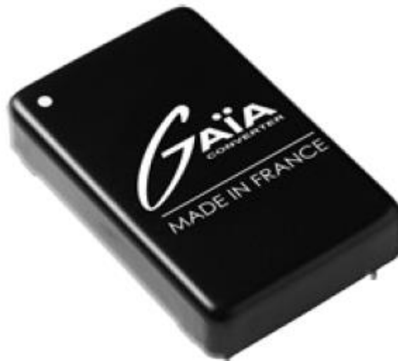
Fig. 3. The HUGD-300, which measures 1 in. x 1.58 in. x 0.5 in., delivers a user-programmable 30-V to 80-V voltage to the hold-up capacitor of a dc-dc converter to increase the stored energy for a given value of capacitance.
