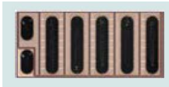
Figure. Housed in a passivated die form, the EPC2018 is a 150-V enhancement-mode GaN-on-silicon FET specifying a maximum R_{DS(on)} of 25 m \Omega with 5 V applied to the gate.
