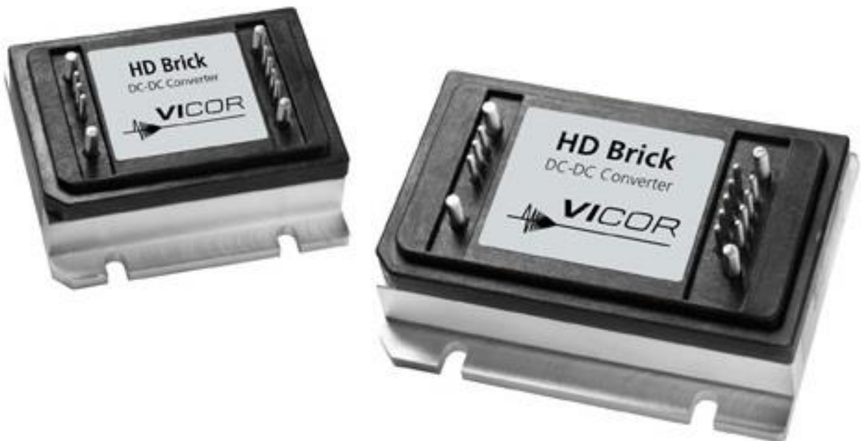
Fig. 2. Offering up to 51% greater power density than competing brick products, the Vicor's HD Brick series's first two standard offerings are a 320-W HD Brick with a nominal 28-V input and a 28-V output in a 48.6-mm x 46.5-mm x 16-mm package, and a 400-W HD Brick with a nominal 300-V input and a 12-V output in a 57-mm x 46.5-mm x 16-mm package.
