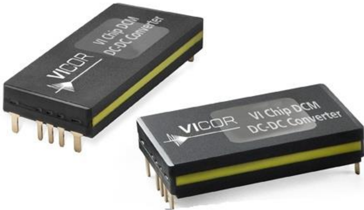
Fig. 1. The ChiP DCM platform spans dc-dc conversion requirements from 12-V to 420-V input and 12-V to 55-V output. This platform includes two pre-configured ChiP DCMs: a 46- x 23-mm 600-W ChiP DCM with a nominal 290-V input and a 13.8-V output; and a 36- x 23-mm 320-W ChiP DCM with a 16-V to 50-V input range and a nominal 28-V output.
