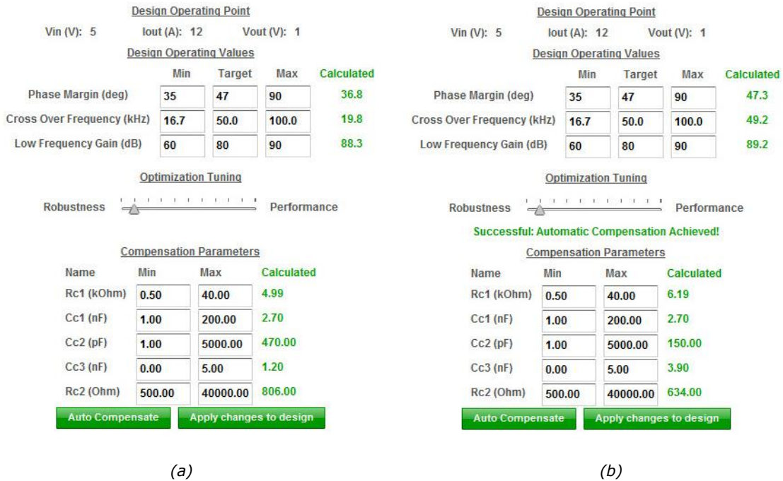
Fig. 4. WEBENCH Compensation Designer allows the user to review existing compensation and stability, and adjust compensation design to new targets. Using the design of Fig. 1 and the larger 1.2- \mu H inductor, the original frequency response summary and compensation components are shown in green type, next to the default targets and ranges (a). With Optimization Tuning slider toward "Robustness," click the button "Apply changes to design." The updated frequency response summary and compensation component values are shown in green type (b).
