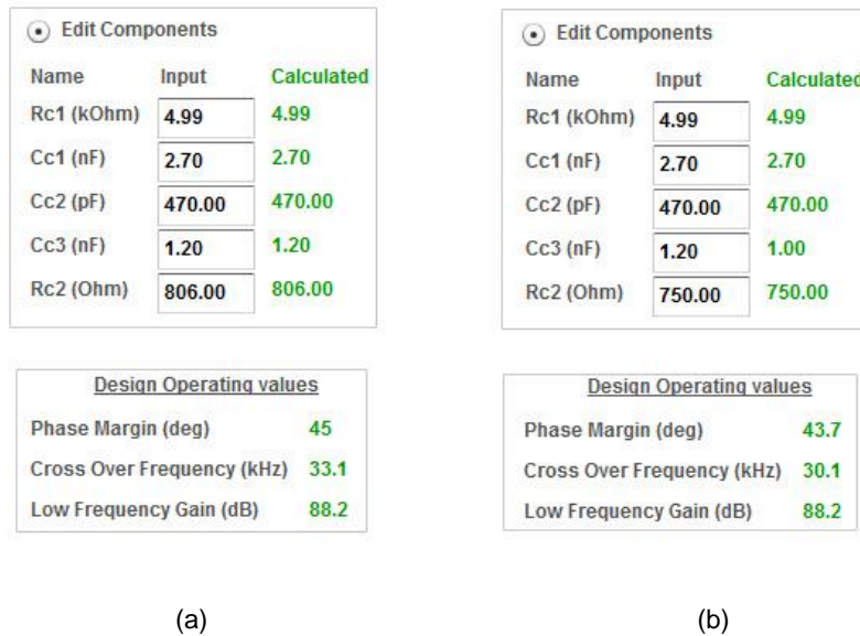
Fig. 9. The starting values for the compensation components are shown in the box on the top left, and the resulting frequency response is shown just below in the box for Design Operating values (a). The result of changing Rc2 from 806 \Omega to 750 \Omega is shown in the box for Design Operating values on the bottom right (b). Notice Cc3 was automatically changed to 1 nF, to partially counter the result of Rc2's change.
