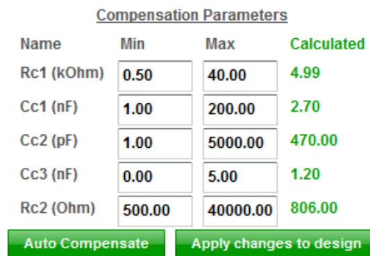
Fig. 10. WEBENCH Compensation Designer allows the user to limit the range of values used for the compensation components.
