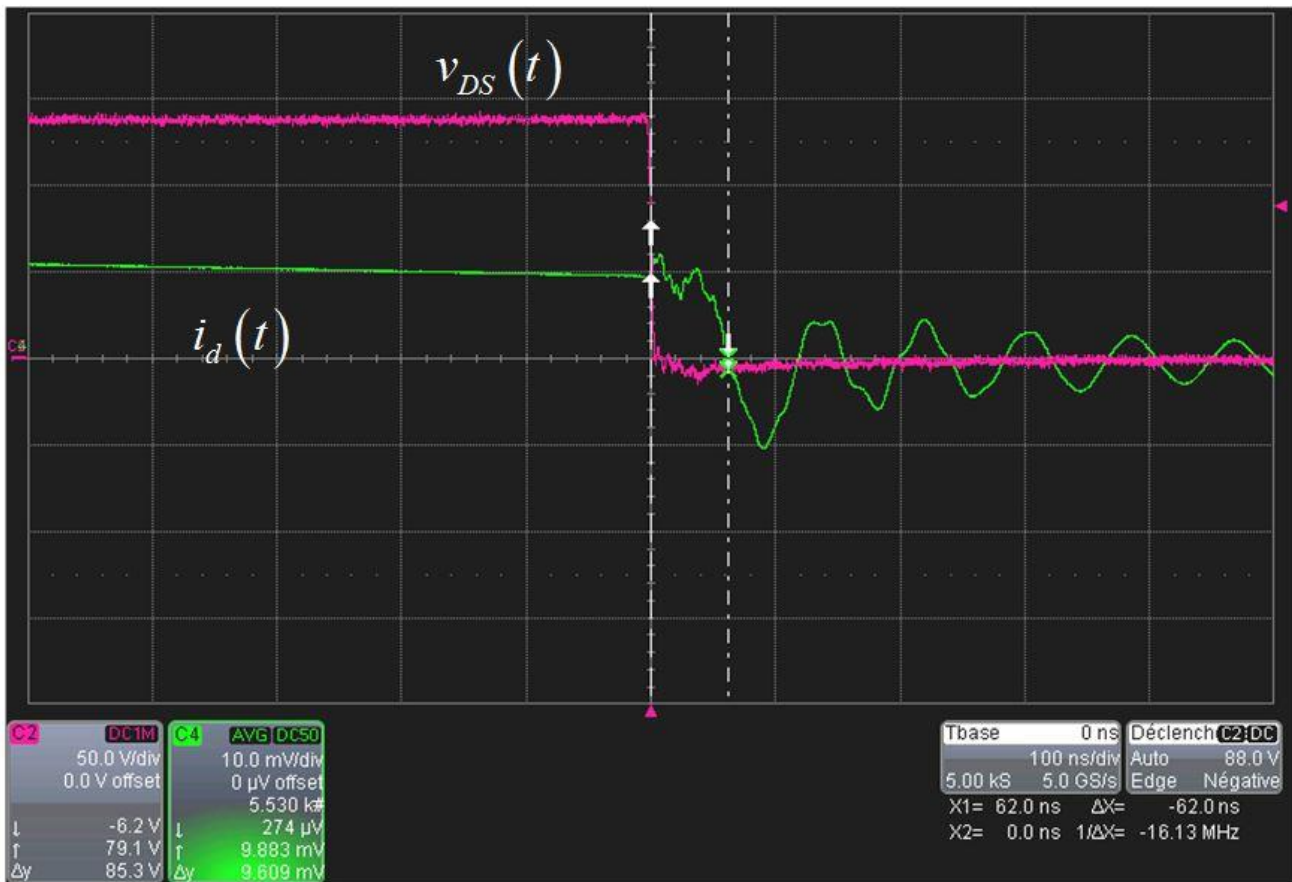
Fig. 10. A close-up of the falling edge shows an extended duration of 62 ns for the secondary-side diode.
