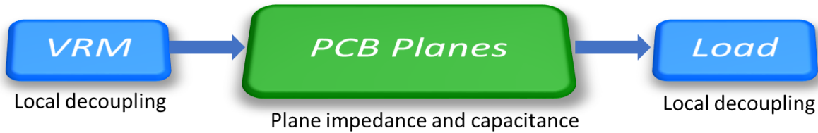
Fig. 1. The power distribution network (PDN) is comprised of the VRM, planes and decoupling capacitors.
