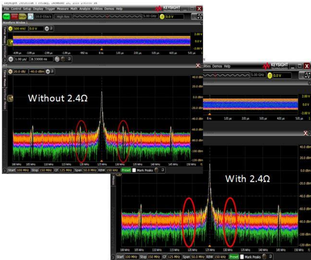
Fig. 4. The clock spectrum shows strong sidebands at 7 MHz without the series resistor present, but these sidebands are eliminated when the series resistor is switched in.
