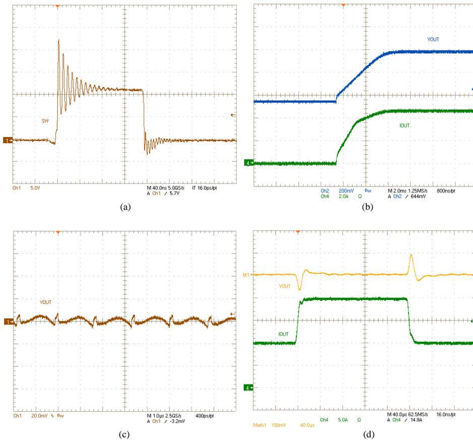
Fig. 6. Performance waveforms at  $V_{IN} = 12\text{ V}$  and  $V_{OUT} = 1.0\text{ V}$ : SW node voltage (a); output voltage monotonic startup with pre-bias (b); output voltage ripple, 20-MHz bandwidth (c); and load transient response, 10 A to 20 A to 10 A at 2 A/ $\mu\text{s}$  slew rate (d).
