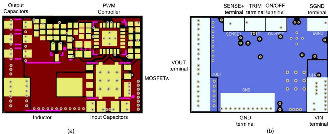
Fig. 3. PCB layout (top down view): top layer (a) and bottom layer (b).
