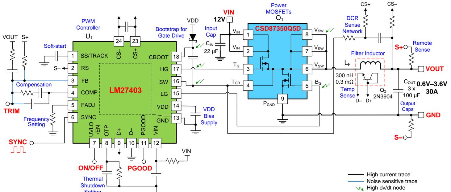
Fig. 2. Synchronous buck converter schematic.
