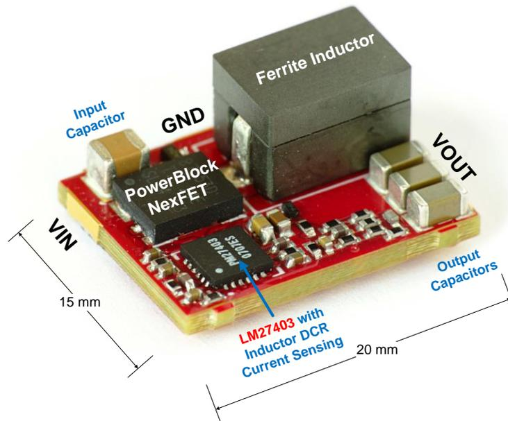
Fig. 4. An implementation a 30-A dc-dc regulator.
