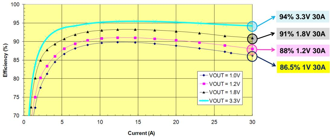
Fig. 5. Converter efficiency vs. load current at various output voltages.  $V_{IN} = 12\text{ V}$  and  $T_{AMBIENT} = 25^{\circ}\text{C}$ .
