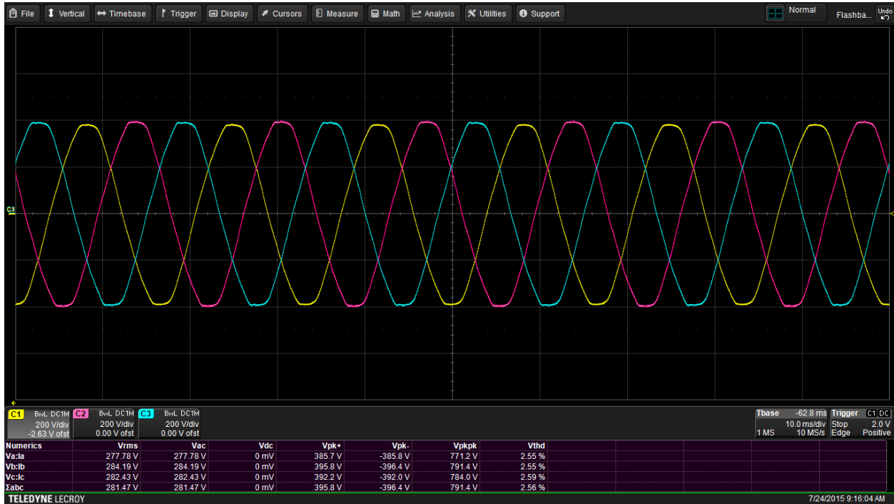
Fig. 9. 480-Vac three-phase line waveforms measured line to neutral.
