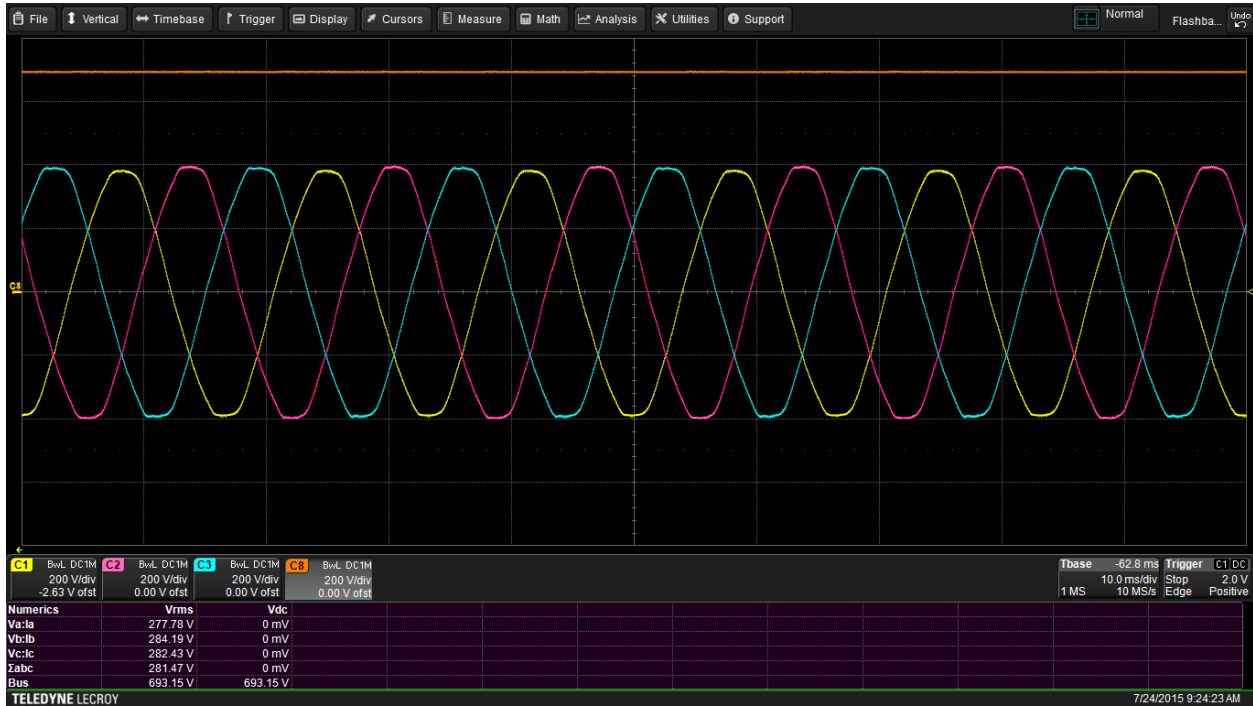
Fig. 12. Applying actual rectification and filtering to the 480-Vac waveforms produces the dc bus voltage measured on channel 8 (orange trace). Its value is 693 V, which is close to the value calculated previously by the Motor Drive Analyzer.
