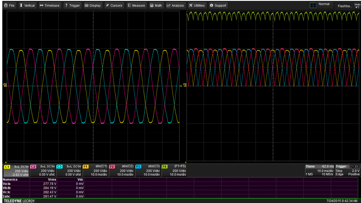
Fig. 11. Probed L-N voltages (left side) and rectified math traces (right side).
