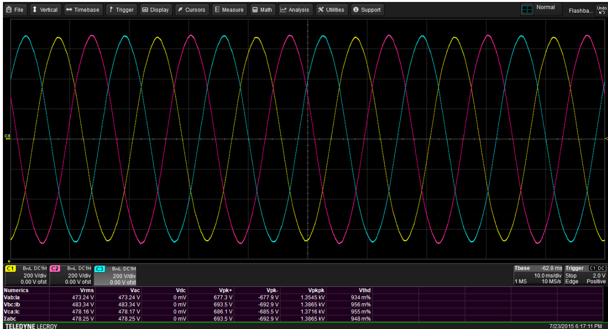
Fig. 5. Waveforms for a 480-Vac three-phase line as measured by a Motor Drive Analyzer and suitably rated voltage probes.
