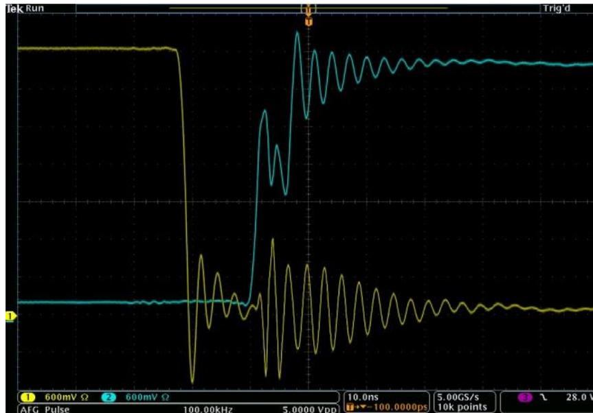
Fig. 11. High-side turn-off, low-side turn-on, and dead time. Ideal waveforms versus actual measurement using IsoVu.
