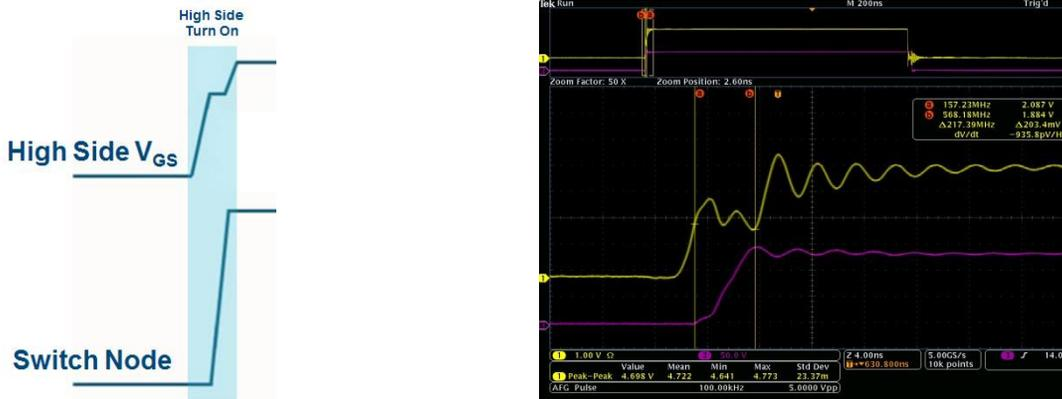
Fig. 9. High-side  $V_{GS}$  turn-on and switch node compared to the ideal.
