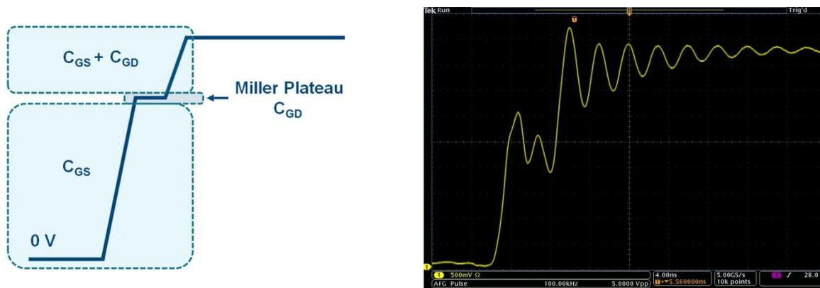
Fig. 7. Comparison of high-side  $V_{GS}$  output as measured using the IsoVu isolated high-voltage measurement system to the ideal.
