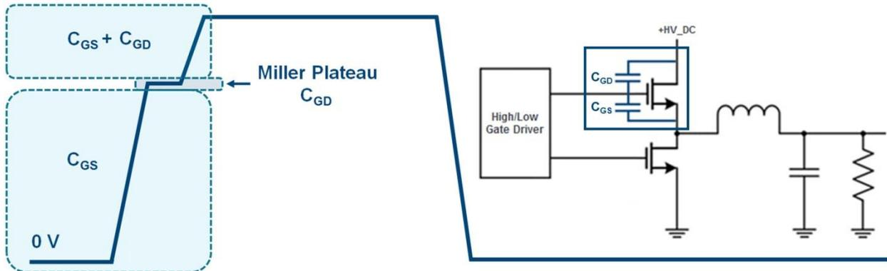
Fig. 3. High-side turn-on characteristics.
