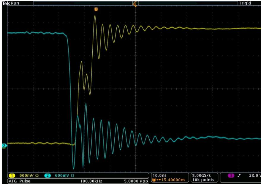
Fig. 10. Interaction of the high-side and low-side switches.
