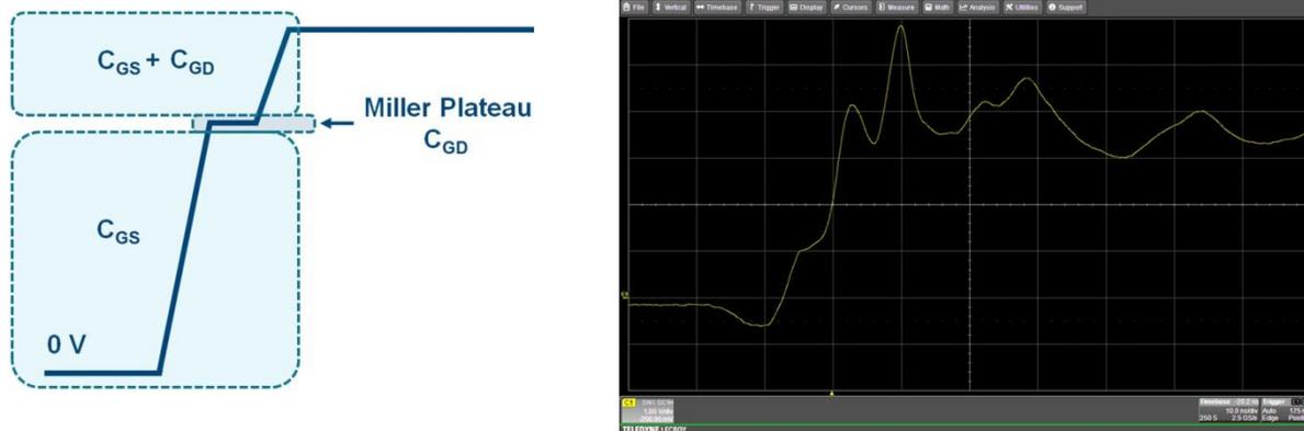
Fig. 4. Comparison of LeCroy's DA1855A high side  $V_{GS}$  output to ideal.
