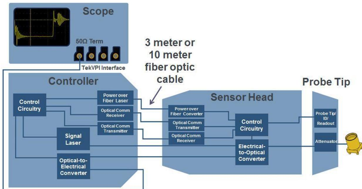
Fig. 6. IsoVu block diagram.
