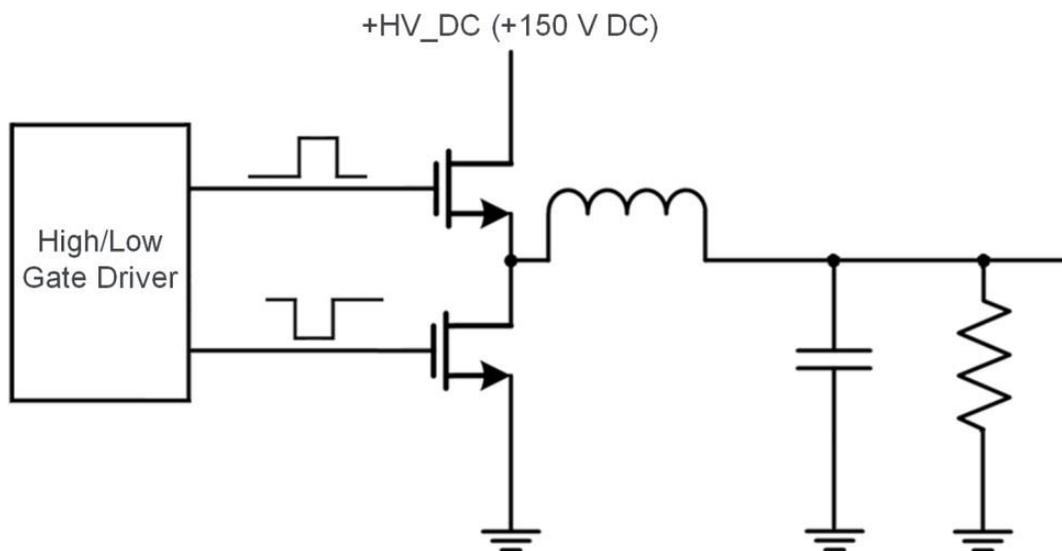
Fig. 1. Half-bridge configuration.
