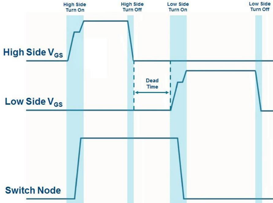
Fig. 2. Example of ideal half-bridge switching waveforms.
