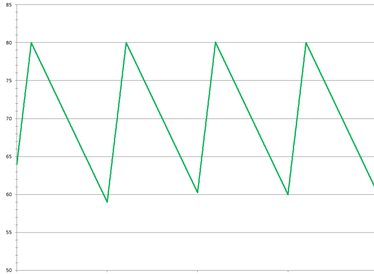
Fig. 2. The current analog of a 20% duty cycle system responding to a large initial perturbation.
