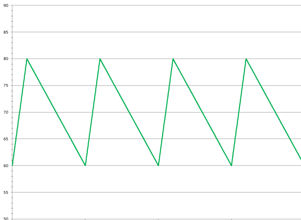
Fig. 1. A current analog waveform for 20% duty cycle operation.
