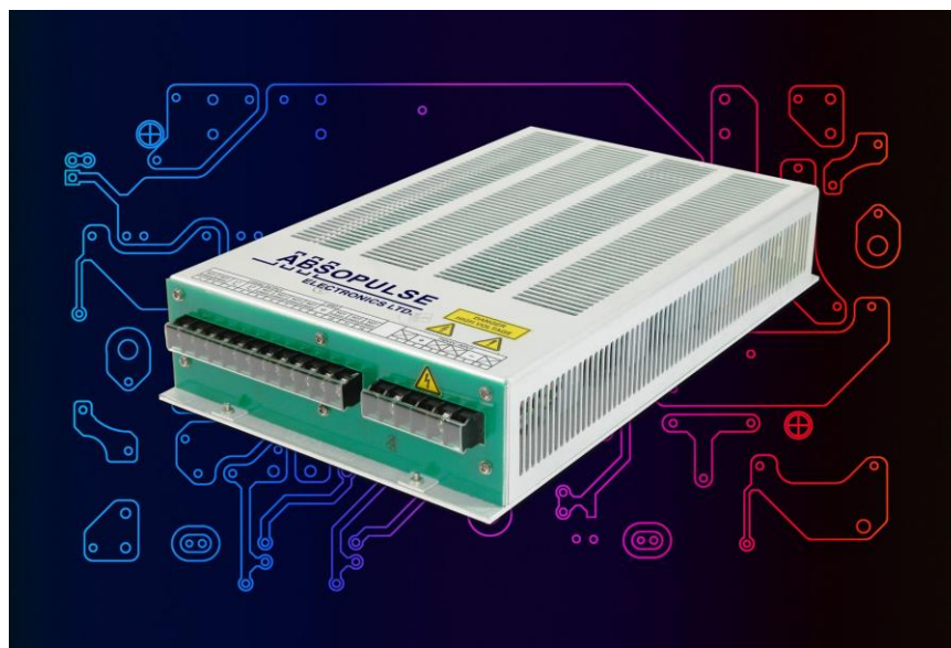
Figure. Featuring a compact 210- x 64- x 365-mm package, the CSH-400-F6 series heavy-duty inverters deliver 400-VA of pure sinewave output at 115 or 230 Vac while operating from a 450-V to 800-Vdc input. These units, which employ conduction and natural convection cooling only (there's no internal fan), are suitable for industrial automation and control, transportation, power plants and electrical utilities.
