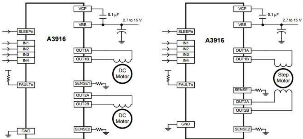
Fig. 1. Requiring just four external components, the A3916 dual DMOS full-bridge motor driver IC is designed for PWM control of low-voltage stepper motors or dual dc motors, delivering up to 1 A per channel. The chip operates from a 2.7-V to 15-V supply.
