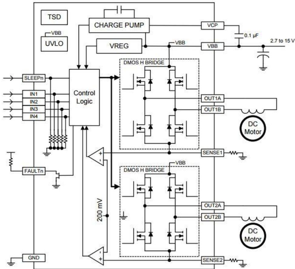
Fig. 2. The A3916 features integrated PWM current control, two DMOS full-bridges with low  $R_{DS(on)}$  outputs; synchronous rectification for reduced power dissipation, an integrated charge pump and on-chip protection such as overcurrent protection, undervoltage lockout and thermal shutdown.
