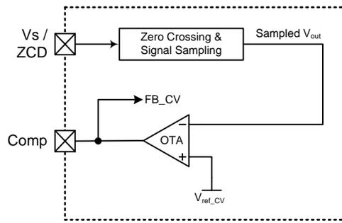
Fig. 5. A simplified schematic for constant-voltage regulation.
