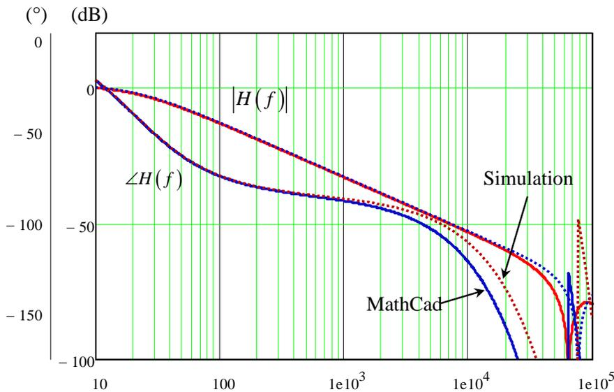
Fig 21. Power stage ac response including the internal ZOH block.
