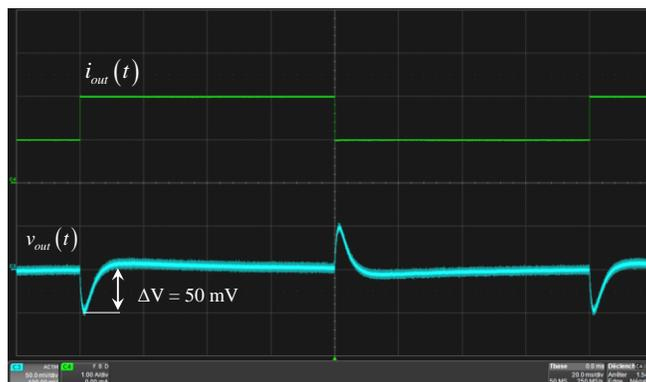
Fig. 27. The transient response measured at low- and high-line conditions confirms the excellent stability of the converter.
