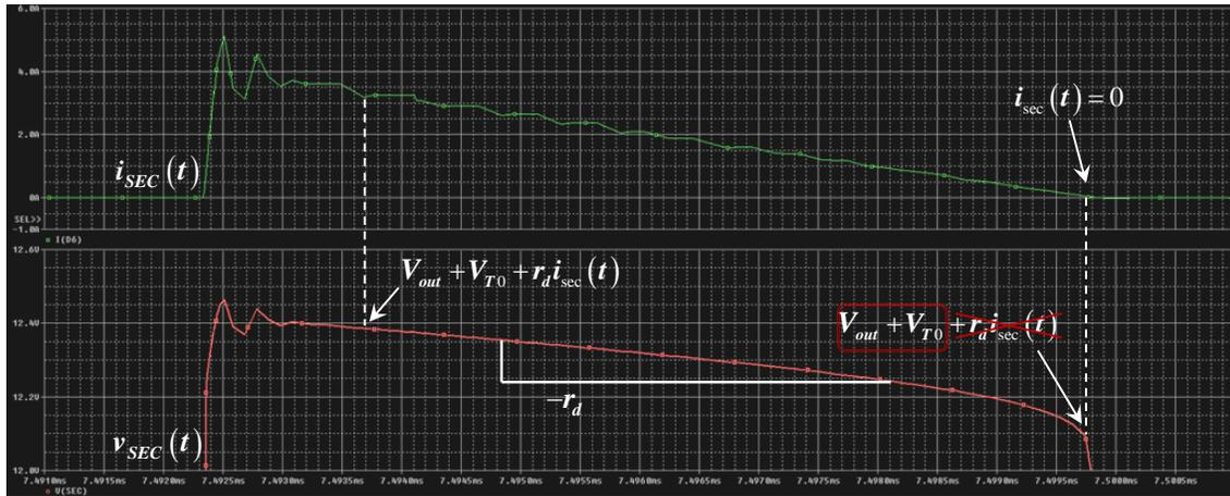
Fig. 4. The effect of diode dynamic resistance on the secondary winding voltage (simulation curves.)
