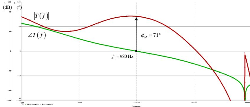
Fig. 25. PSpice open-loop gain of the BCM flyback converter operated in PSR mode
