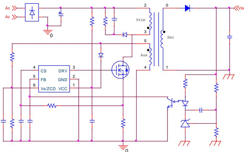
Fig. 1. Simplified schematic of a classical flyback structure.
