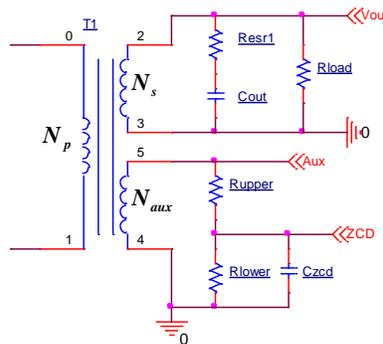
Fig. 11. The transformer and secondary components. Simplifying this schematic will allow us to simply the power stage average model.
