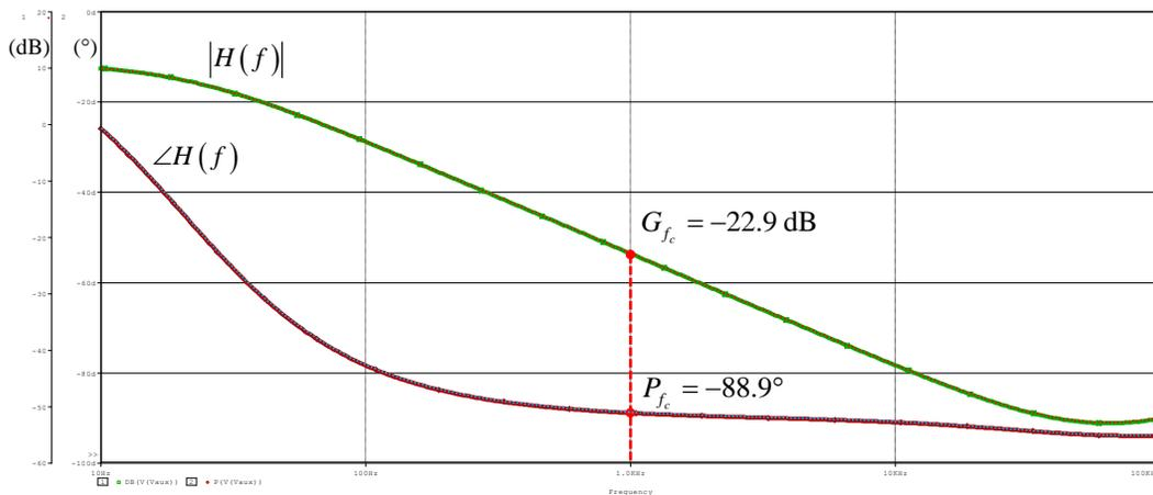
Fig. 15. Transfer function (Ctrl node to Vaux) obtained with the simplified schematic.
