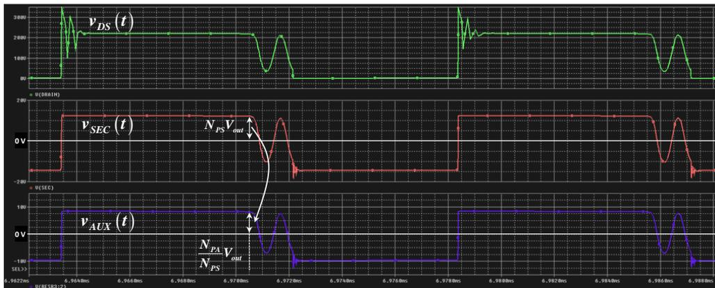
Fig. 3. SPICE waveforms measured on or near the flyback transformer.
