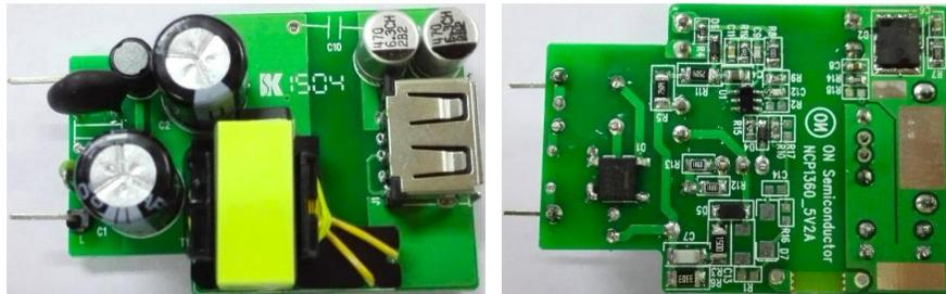
Fig. 26. A PSR board using ON Semiconductor's NCP1365 has been assembled. It delivers 5 V and up to 2 A of output current.
