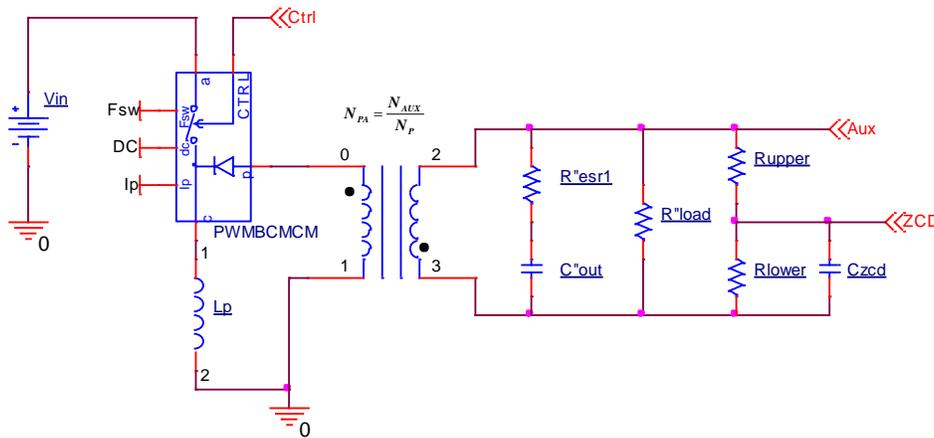
Fig. 14. Simplified PWM switch model.
