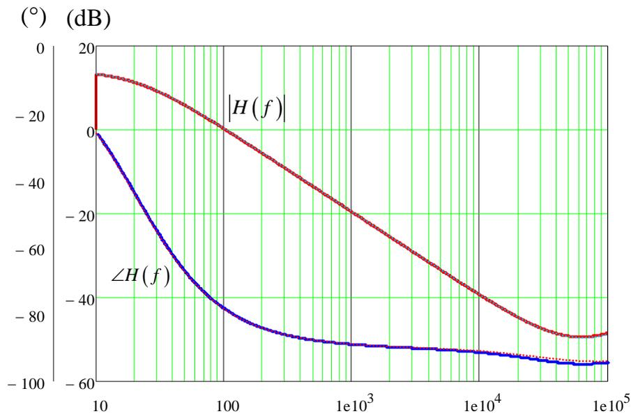
Fig. 20. Power stage transfer function plots generated using Mathcad.
