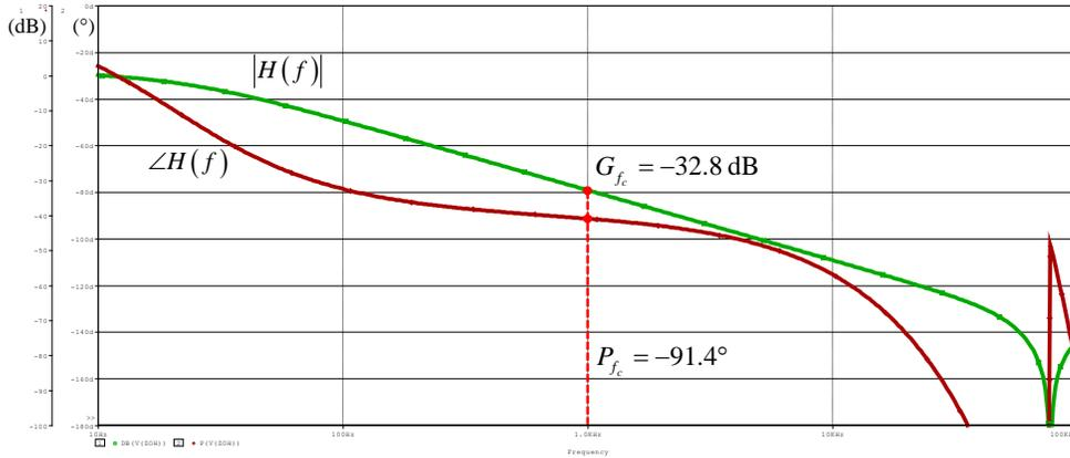
Fig. 18. Transfer function of the power stage now including the internal sample-and-hold network.
