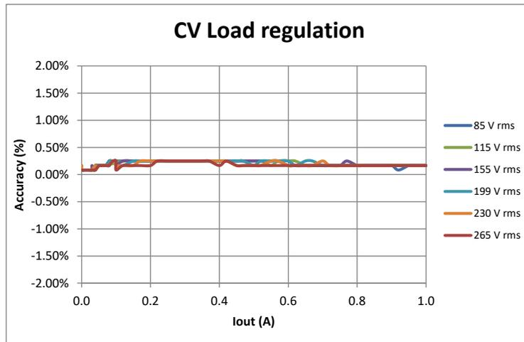
Fig. 7. Constant voltage regulation as a function of load current and input voltage for a PSR controller measured in the lab.
