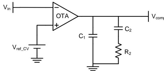
Fig. 22. OTA with type-2 compensation.
