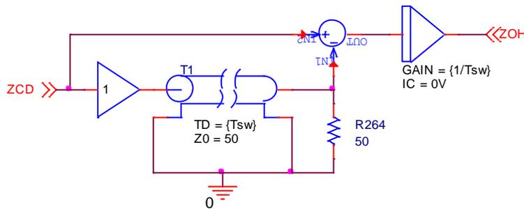
Fig. 16. ZOH modeling with delay line plus an integrator.
