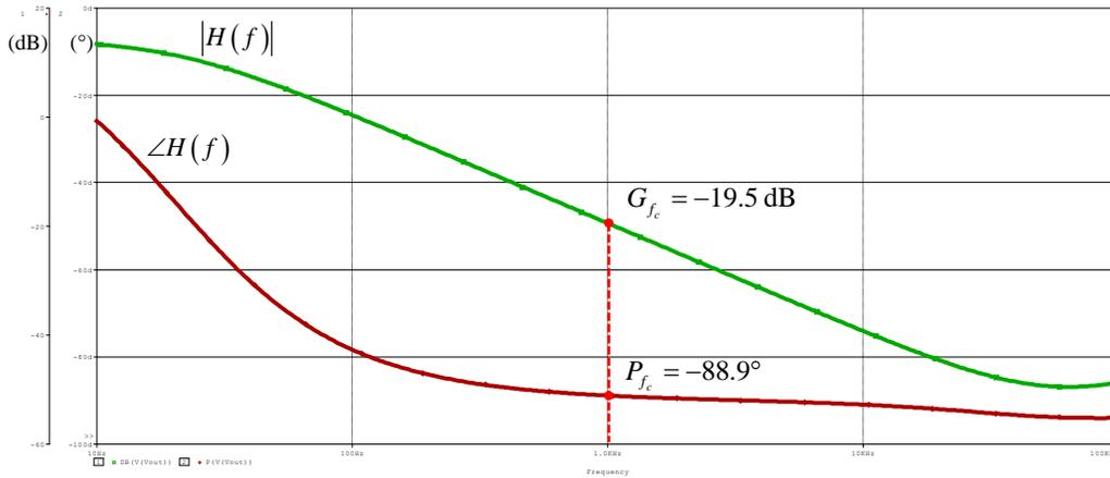
Fig. 9. Power stage transfer function.
