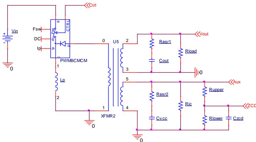
Fig. 8. The PWM switch model in a flyback converter.
