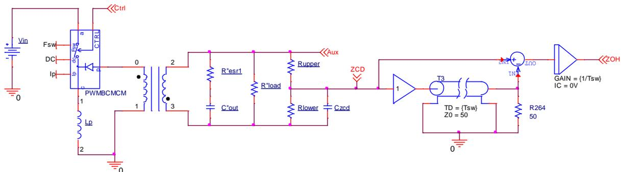
Fig. 17. Average model of the power stage including the sample-and-hold network.
