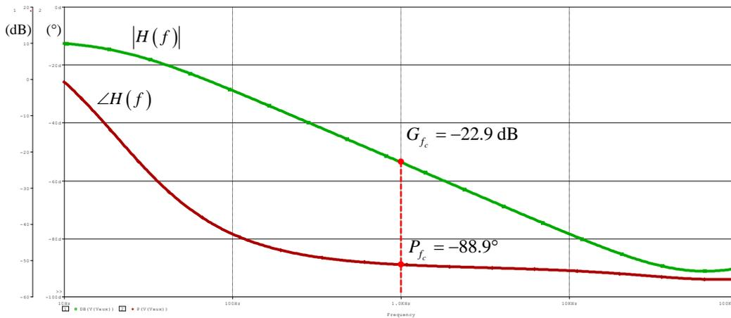
Fig. 10. Transfer function observed on the auxiliary winding.
