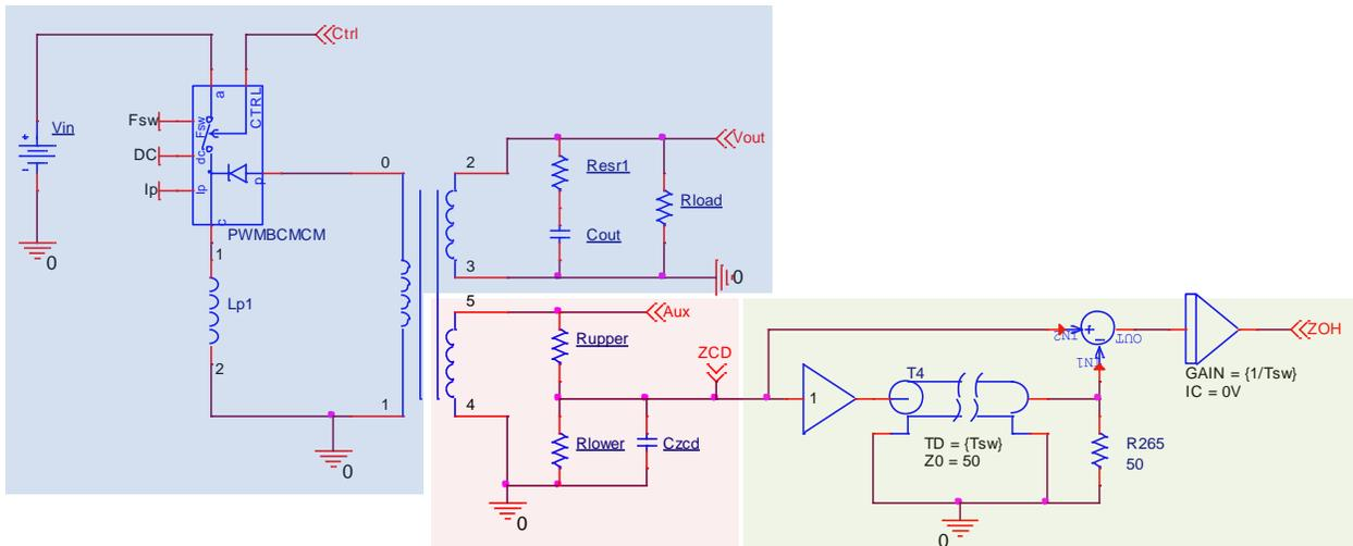
Fig. 19. The power stage is divided into three main sections—the power stage, the auxiliary winding structure, and the sample-and-hold network.
