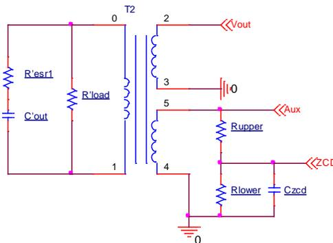
Fig. 12. Output capacitor and load reflected to the primary side.
