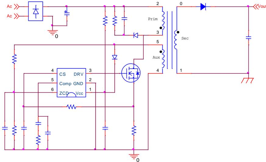
Fig. 2. Simplified schematic of a PSR-based flyback structure.
