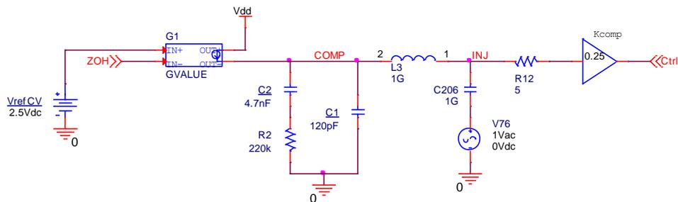
Fig. 24. Type-2 compensation schematic with the internal  $K_{comp}$  divider.
