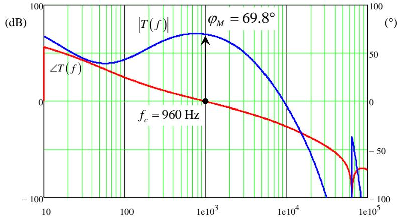
Fig. 23. Ac response generated in Mathcad for a converter with a type-2 compensation network.
