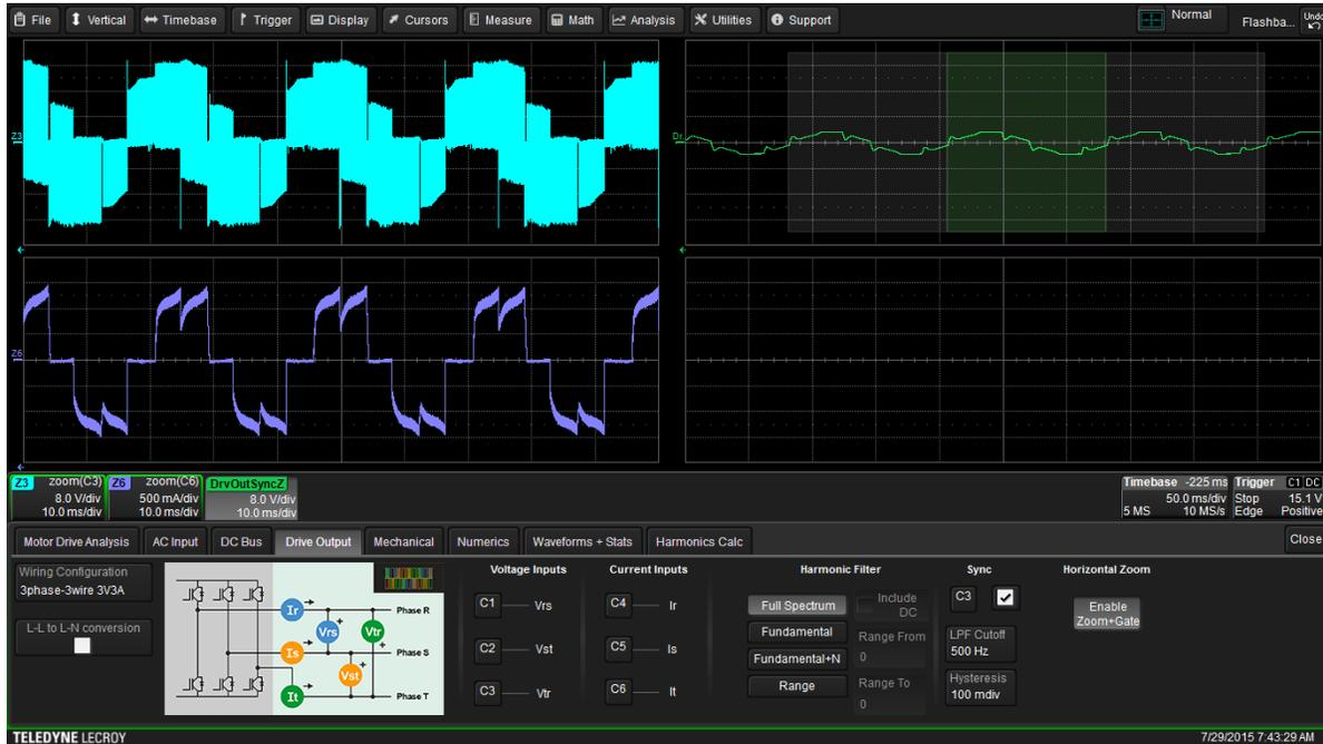
Fig. 8. Even with the low-voltage BLDC six-step commutated drive output line-to-line voltage (Z3, light blue, upper left) measured here, we can still obtain an accurate Sync signal from this line-to-line voltage signal using the default settings for the low-pass filter and hysteresis. The filtered Sync signal with cyclic period overlays appears as DrvOutSyncZ (green, upper right).
