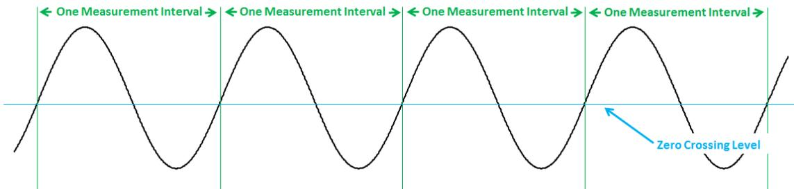
Fig. 2. Cyclic period measurement intervals on a sinewave signal. Determining the measurement interval is simple in this case.
