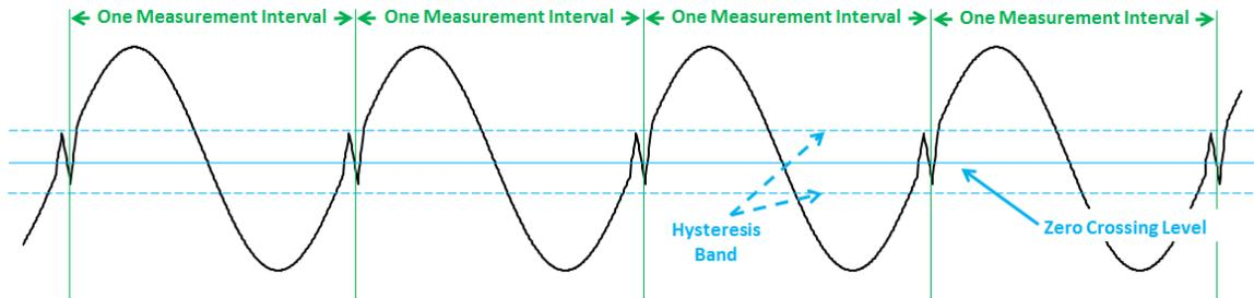
Fig. 4. Setting a hysteresis band corrects for non-monotonicity when measuring intervals.
