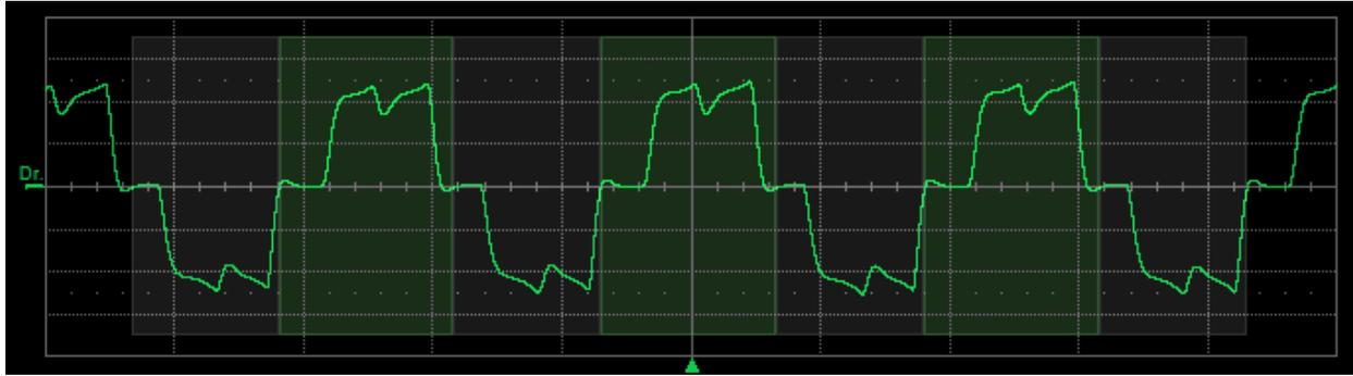
Fig. 10. This line current signal is essentially the same as in Fig 9, but the presence of slightly more noise causes the MDA to determine the cyclic period to be just half of the actual period as the overlays indicate when the default setting for hysteresis band is used.
