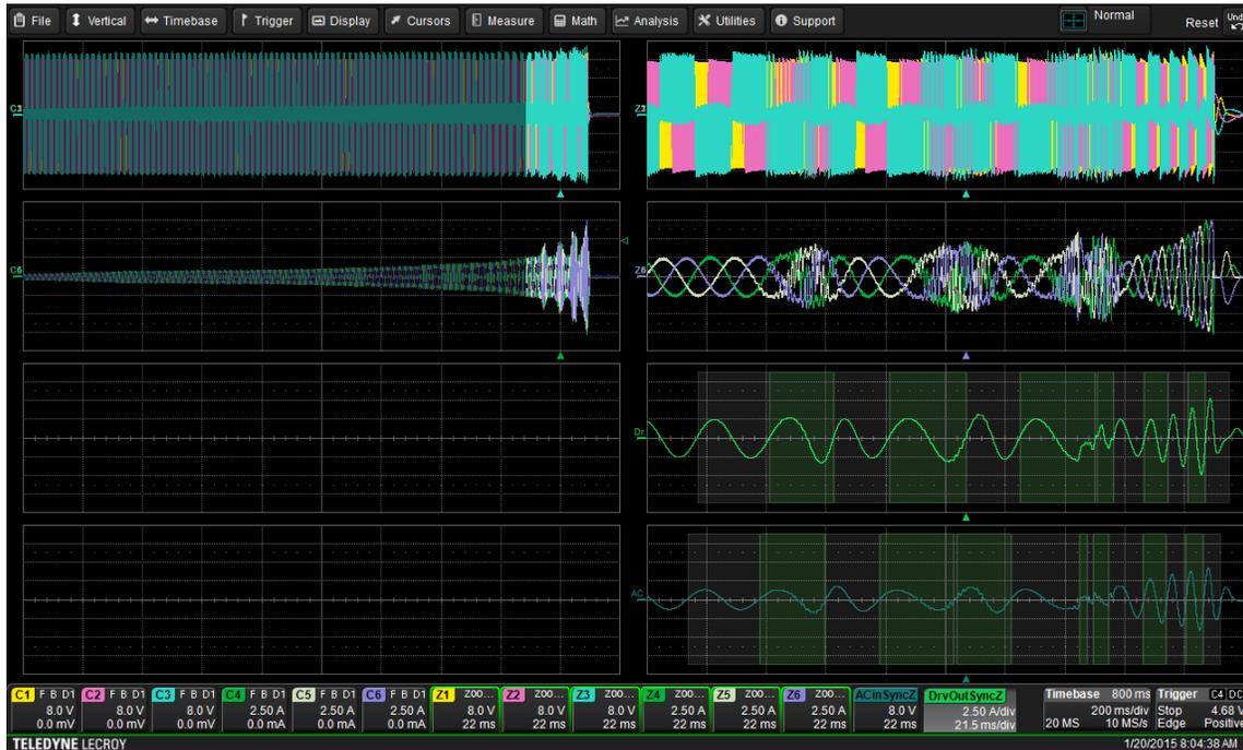
Fig. 17. Adjusting filters reveals DriveOutSyncZ (C4, second waveform from the bottom on the lower right) is the better choice as the Sync signal.
