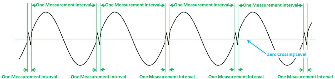
Fig. 3. A non-monotonic signal produces “false” measurement intervals.
