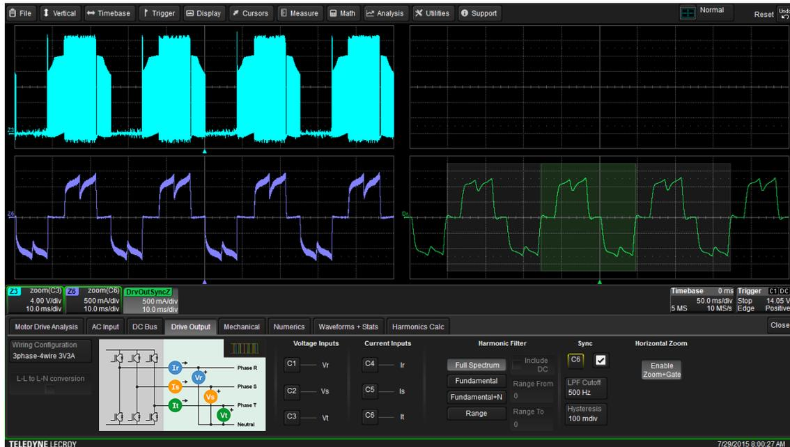
Fig. 12. When the line-current waveform is selected as the Sync signal, the MDA is able to correctly determine the cyclic period using default settings.
