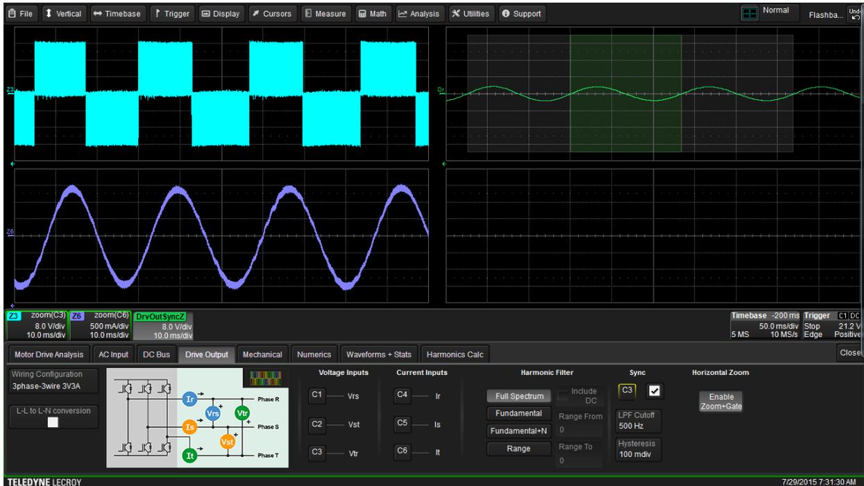
Fig. 6. A single line-to-line voltage (Z3, light blue, upper left) and line-current output (Z6, purple, lower left) of a low-voltage vector FOC drive. The filtered Sync signal with cyclic period overlays appears as DrvOutSyncZ (green, upper right.)
