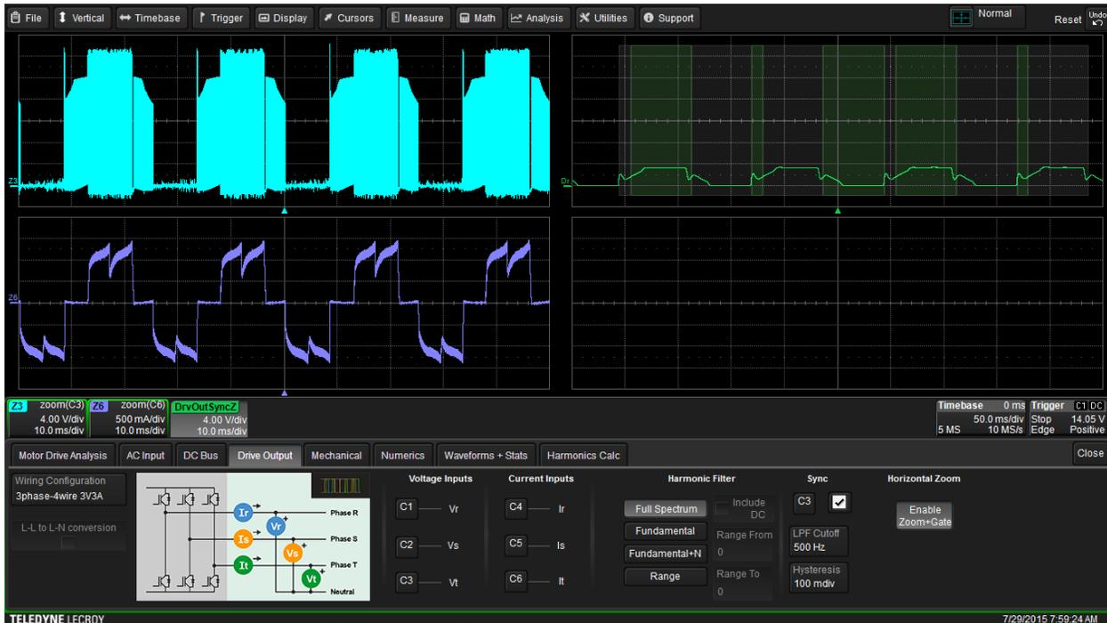
Fig. 11. A line-to-reference voltage (Z3, light blue, upper left) of a low-voltage, BLDC, six-step commutated drive output is chosen as the Sync signal, but the MDA software cannot accurately determine the cyclic period.
