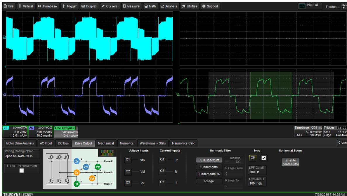
Fig. 9. Choosing the line-current signals as the Sync signal for the low-voltage BLDC six-step commutated drive output produces similar results to those obtained in Fig. 8.
