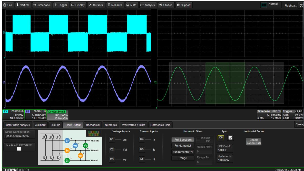
Fig. 7. Using the line current signal (Z6, purple, lower left) as the Sync signal, we can make the same cyclic period determination as when we used the line-to-line voltage signal but filtering is not required. The Sync signal appears on the lower right.
