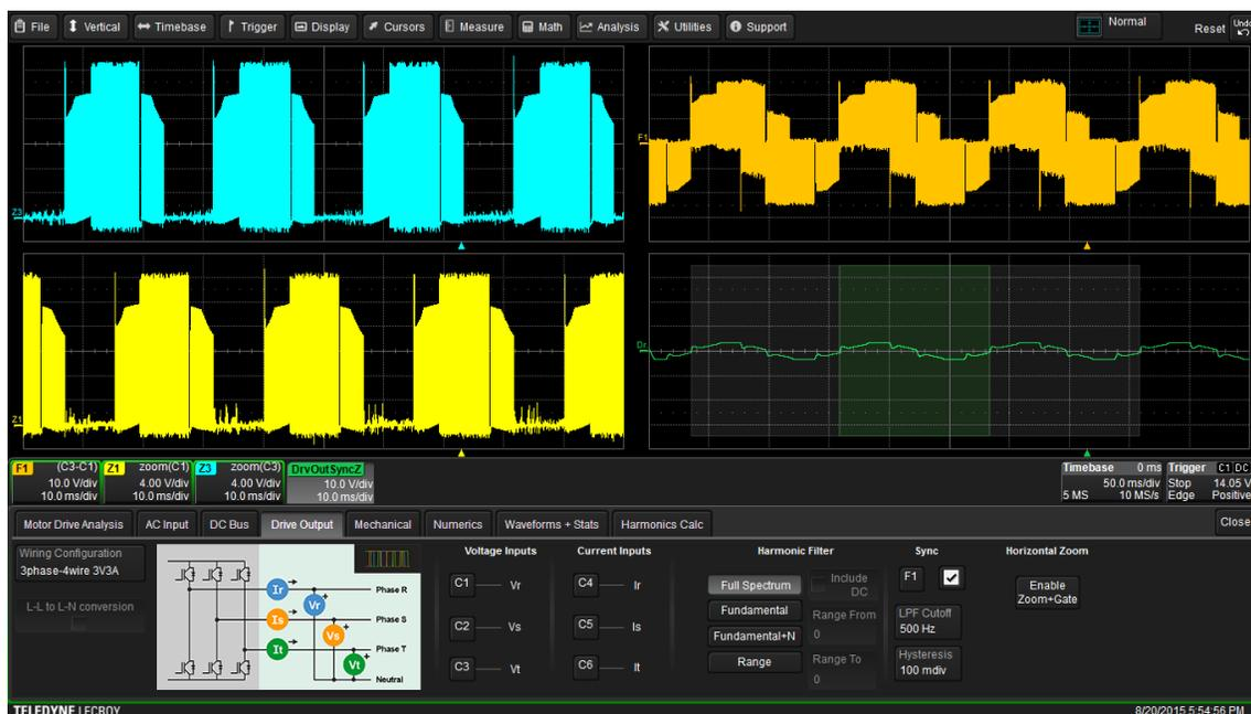
Fig. 13. A Math function within the MDA takes the difference between the two line-to-reference waveforms shown on the left and uses this difference waveform as the Sync signal shown on the lower right.
