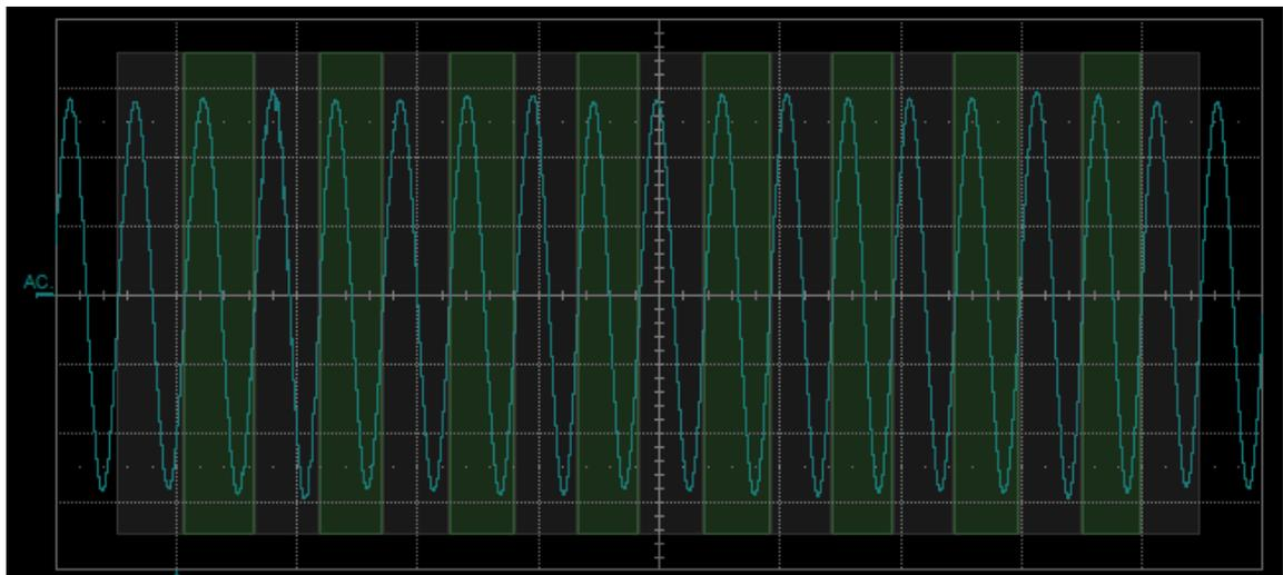
Fig. 5. Colored overlays mark the measurement cycles on Sync signal.
