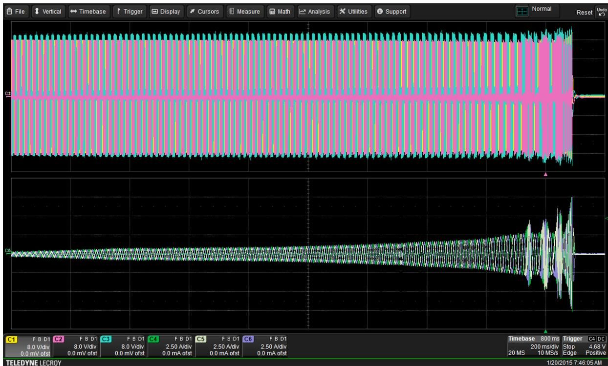
Fig. 14. Initial display of input source waveforms for a sine-modulated, three-phase drive.
