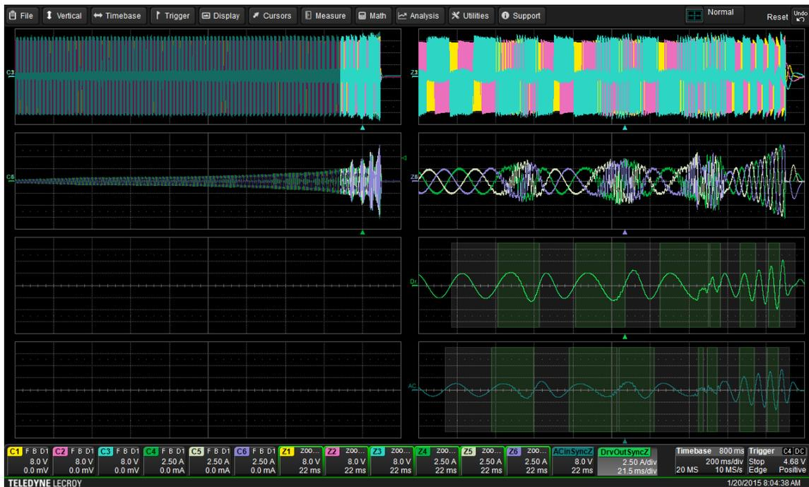
Fig. 16 Changing zoom position changes display of all zoomed waveforms, including Sync signals.
