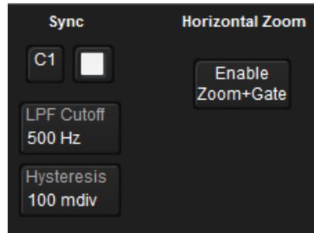
Fig. 1 Setup for the Sync signal in the Teledyne LeCroy's Motor Drive Analyzer.
