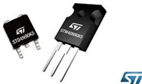
Figure. The 900-V MDmesh K5 super-junction MOSFETs are said to be the first 900-V MOSFETs with on-resistance below 100 m \Omega and the best R_{DS(ON)} among DPAK devices. Also, claiming the lowest gate charge ( Q_g ), these devices promise faster switching for greater flexibility where a wide input-voltage range is required.
