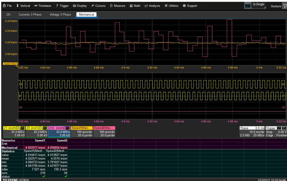
Fig. 27. Angle tracking observer applied to QEI digital signals.
