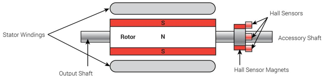
*Fig. 9. Magnetic fields produced by Hall sensor magnets embedded in the rotor are sensed by Hall sensors mounted to an assembly surrounding the rotor. The electrical signals produced by the Hall sensors permit the control system to determine rotor location and speed.*
