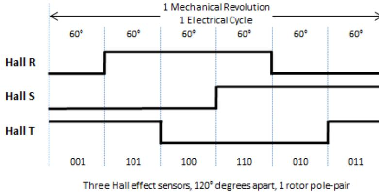
Fig. 10. In the BLDC motor of Fig. 9, one of the Hall-effect sensors makes a positive transition every 120°. In the case of a motor with a single rotor-pole pair, one electrical cycle completes in the same time as one mechanical shaft revolution.
