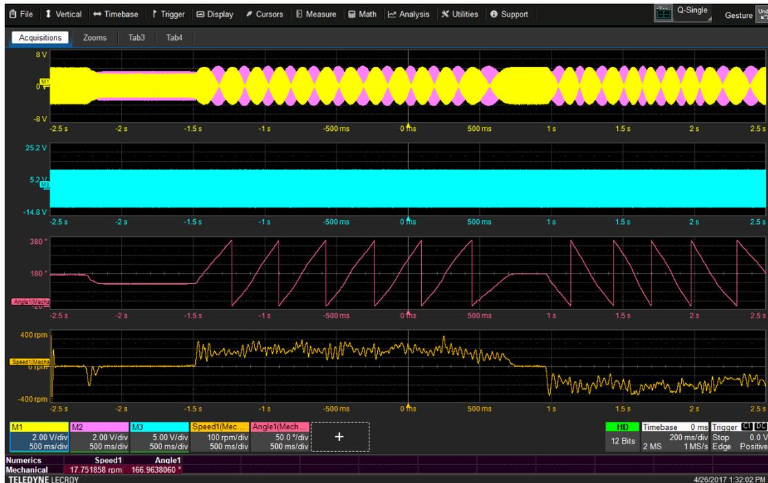
Fig. 8. Capture of resolver signals measuring the dynamic movement of a servo motor shaft. Resolver sine (M1, yellow), cosine (M2, magenta), and excitation frequency (M3, or light blue) are shown along with speed and angle mean values and waveforms.
