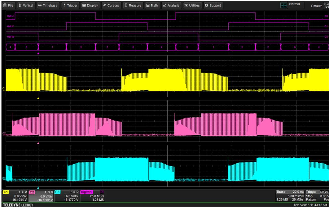
Fig. 12 Hall-effect sensor signals (Digital 1, purple trace) and line-to-reference voltage output envelopes (C1, or yellow trace, C2, or magenta trace, and C3, or blue trace) are shown for the BLDC motor measured in Fig. 11.
