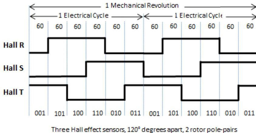
Fig. 15. With two rotor-pole pairs, two electrical cycles of the Hall effect signals will be completed in one revolution of the motor shaft.
