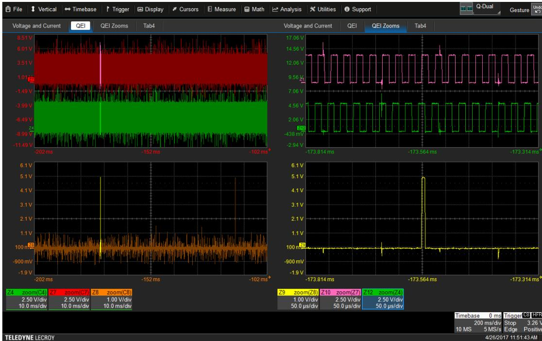
Fig. 20. A, B, and Z signals from a QEI acquired using the analog channels of an MDA. 100-ms acquisitions of these signals are shown on the left side of the display and zoomed versions (over 0.5 ms) are shown on the right side.
