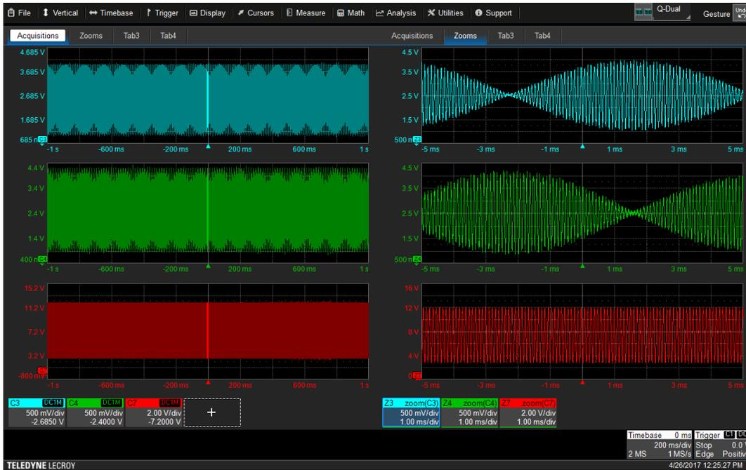
Fig. 4. Measurement of resolver signals using the Motor Drive Analyzer. On the left side of the display, we see full 2-s acquisitions of the excitation reference (C7, bottom left), the sine output (C3, top left) and cosine output (C4, middle left). Zooms of the full acquisitions appear on the right.
