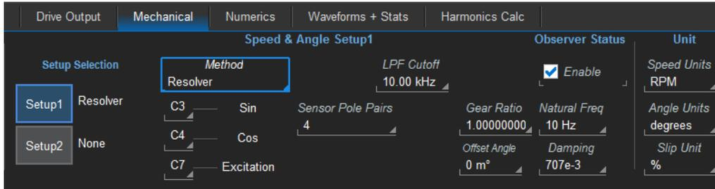
Fig. 7. The MDA is configured for converting resolver data to speed and angle values with the angle tracking observer filter enabled.
