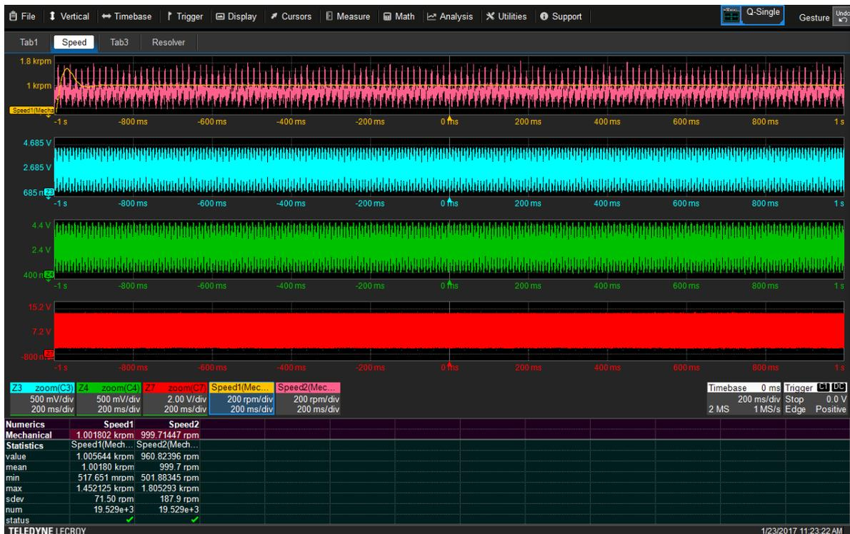
Fig. 30. Angle tracking observer applied to Resolver signals for full 2-s acquisition. This longer capture highlights the filter start-up time.
