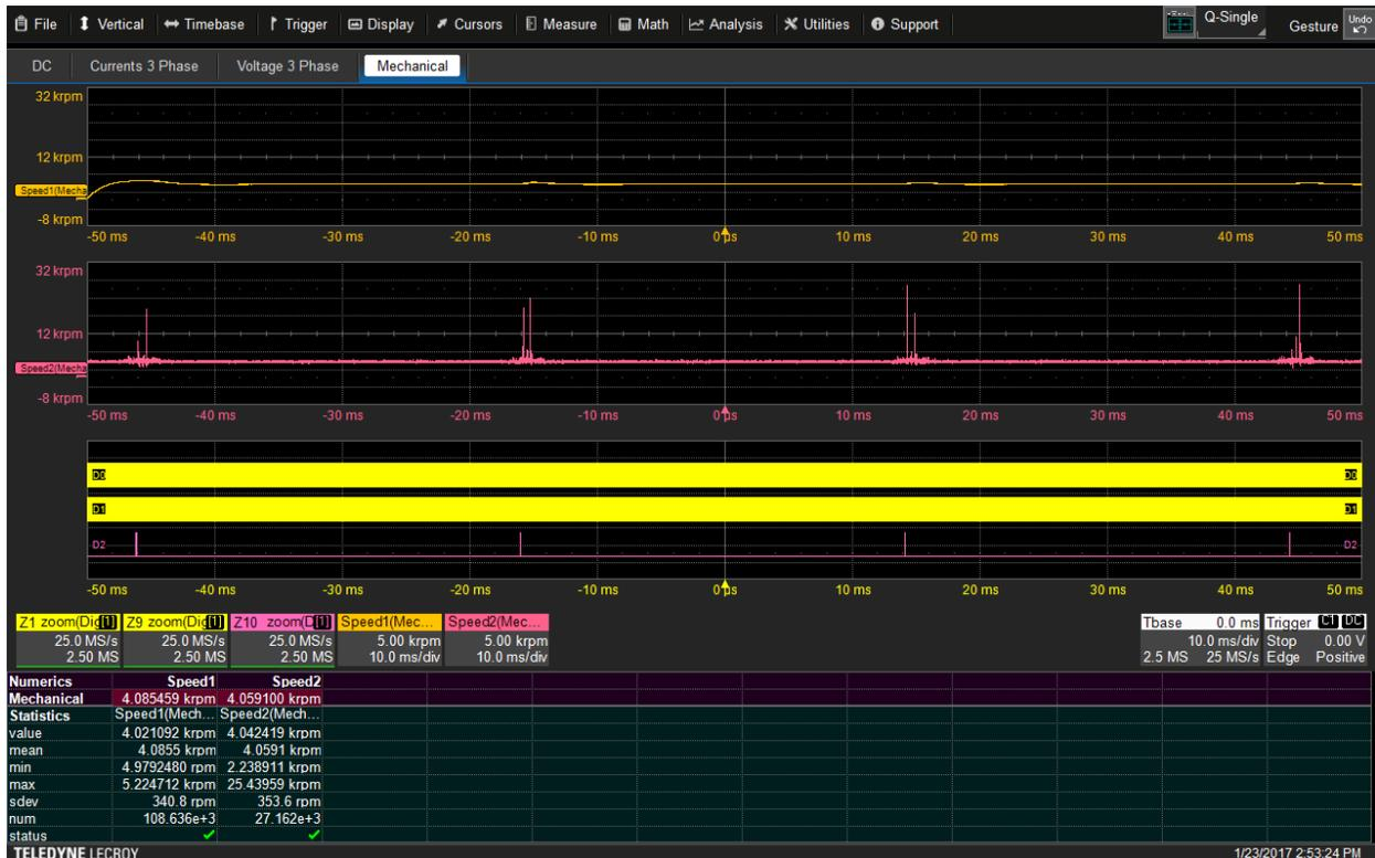
Fig. 28 Angle tracking observer applied to QEI digital signals for full 100-ms acquisition.
