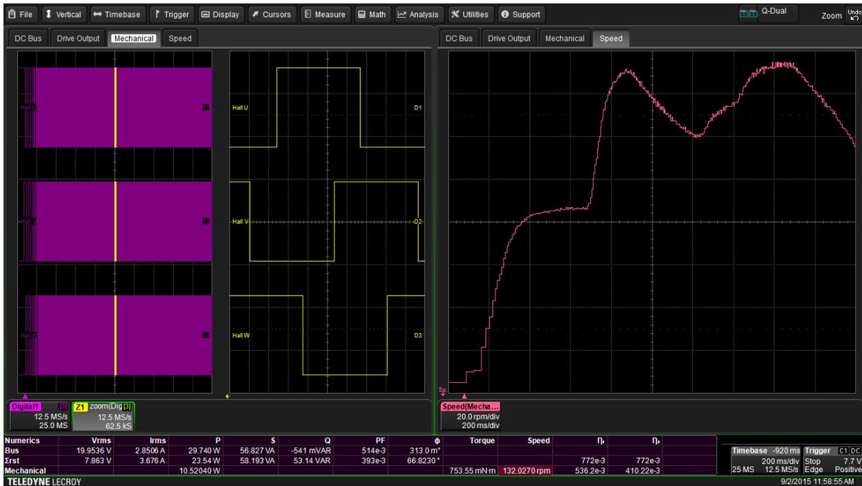
Fig. 16. Hall effect sensor signals (shown on the left) captured by the MDA are used to calculate the speed of the rotor.
