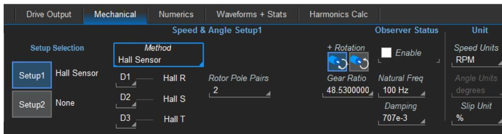
Fig. 18. Configuration of MDA settings for calculating motor speed from Hall sensor data.
