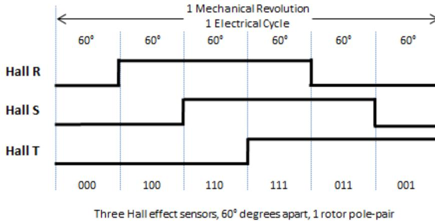
Fig. 14. Hall effect sensors may be placed 60 degrees apart. As was the case with the more widely spaced sensors, one electrical cycle is completed in the same time as one mechanical shaft revolution when there is a single rotor-pole pair.
