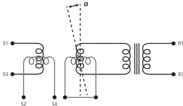
Fig. 2. A resolver generates two sine wave signals that are 90° apart. These signals can be used to determine shaft speed and angle.
