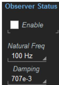
Fig. 25. Configuring the MDA for use of the Angle Tracking Observer algorithm.
