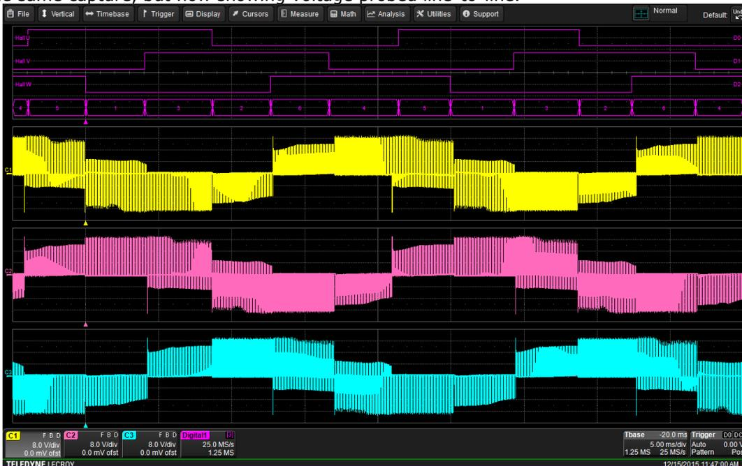
Fig. 13. Hall-effect sensor signals and voltage output envelopes are measured again, but with the voltage probed line-to-line.
