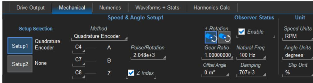
Fig. 23. Configuration of MDA settings for calculating motor speed and angle from QEI data.
