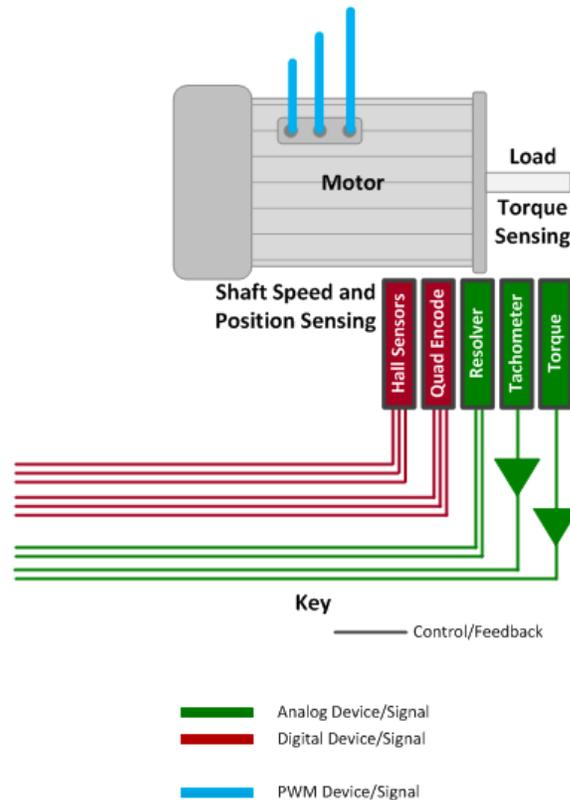
Fig. 1. Motors use a variety of sensor types to measure torque, speed, position, and rotational direction of the motor shaft.
