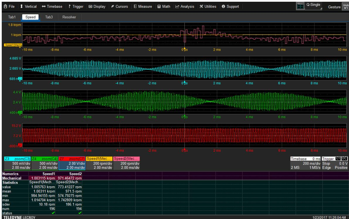
Fig. 29. Angle tracking observer applied to resolver signals for short (20-ms) acquisition.
