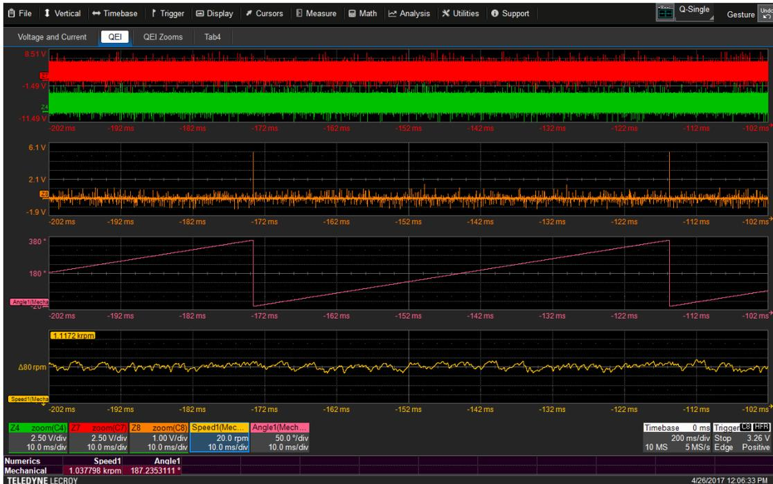
Fig. 21. The MDA calculates speed and angle values from QEI signals, displaying the results as waveforms as well as values in the Numerics table.
