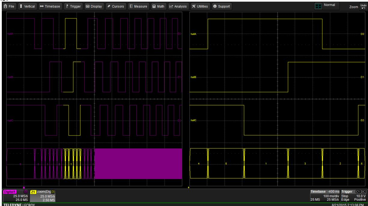
Fig. 11. Hall-effect sensor signals produced by a BLDC motor like that depicted in Fig 9 (one rotor-pole pair) are captured using the digital logic inputs of the Motor Drive Analyzer. The waveforms on the left (Digital1, purple) are the full 2-s captures of the three Hall-effect sensor signals, and the images on the right are zoomed versions of these signals.
