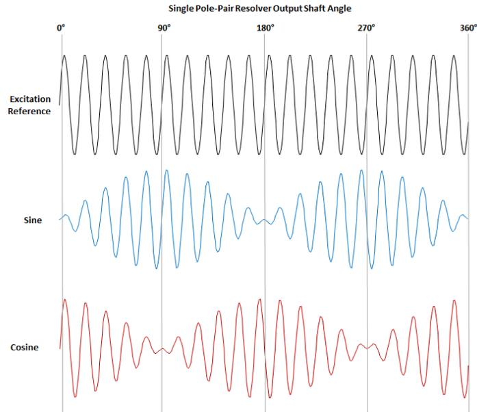
*Fig. 3. A basic resolver with a single pole pair generates sine and co-sine outputs. One complete transition of the sine and co-sine waves represents a single rotation of the shaft. The rotor shaft angle (position) is calculated from the arctangent of the ratio of sine and cosine amplitudes.*
