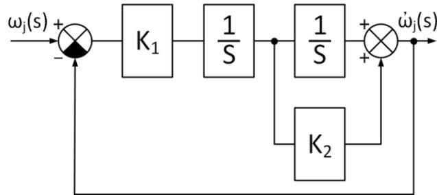
Fig. 24. An angle tracking observer implements the transfer function shown here in software.
