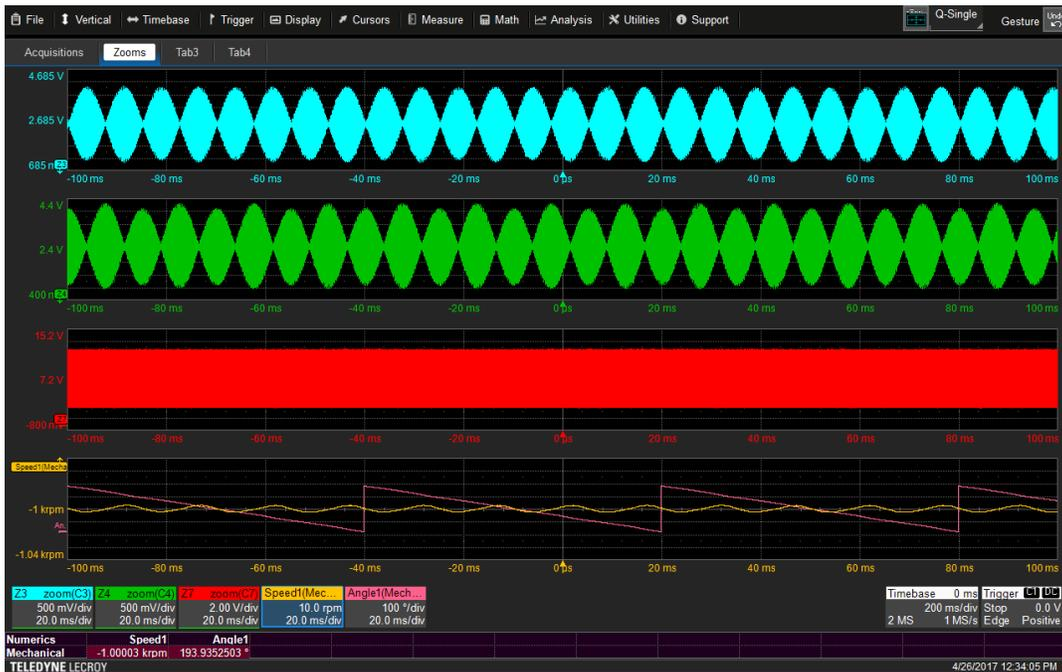
Fig. 5. The MDA calculates speed and angle values from the captured resolver waveforms.
