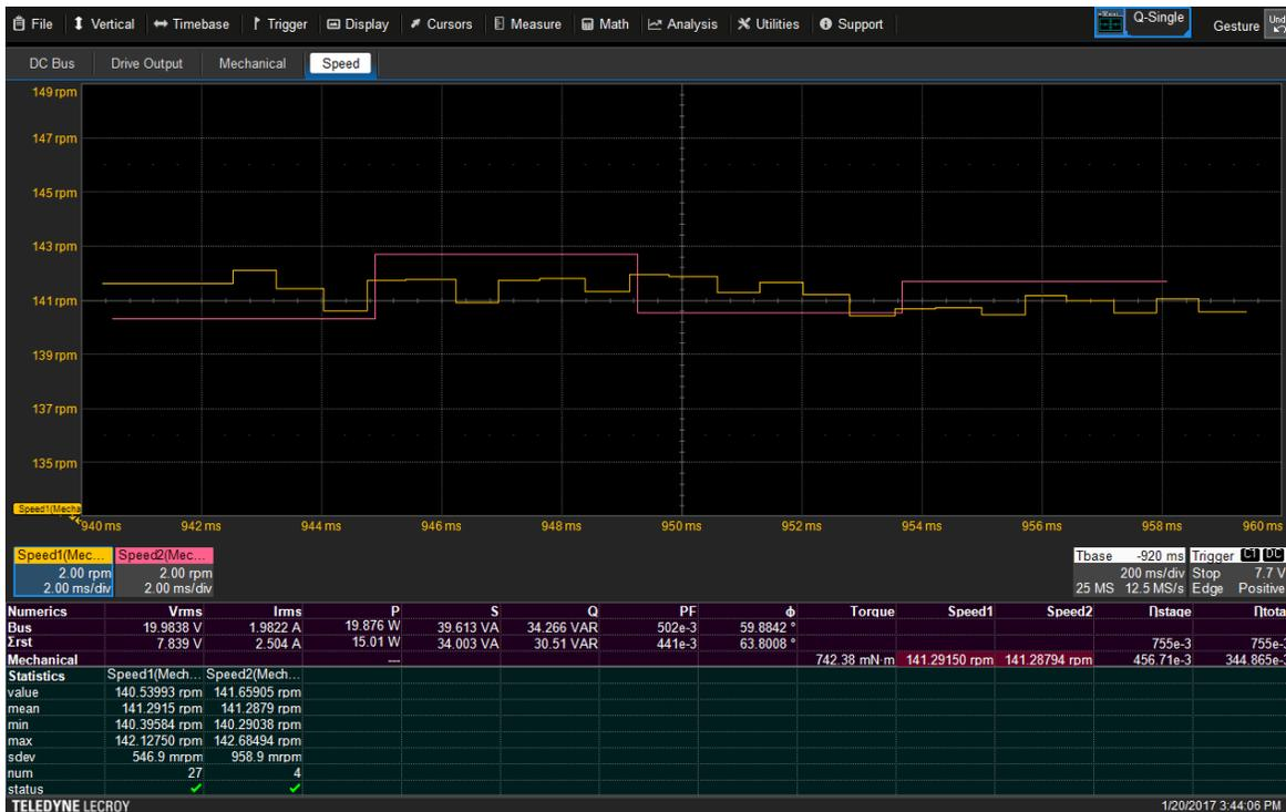
Fig. 26. Angle tracking observer applied to Hall sensor digital signals.
