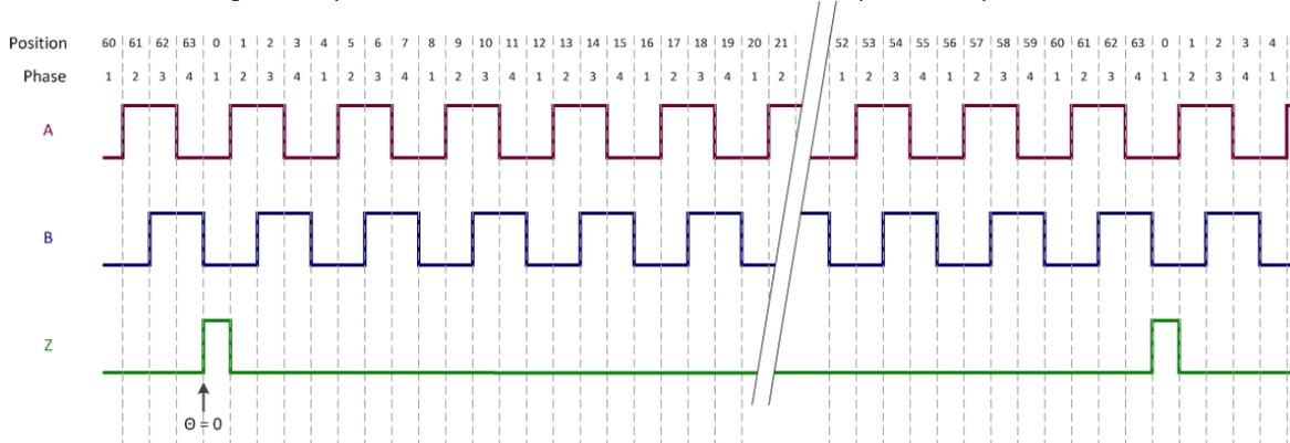
*Fig. 19. With a QEI, the three digital pulses (A, B and Z, or the Index pulse) are used to define speed, direction and absolute position of the rotor. The A and B, which are 90° out of phase ("in quadrature") communicate a two-bit pulse sequence N times per shaft revolution. The Z index pulse signal is used to communicate position information once per revolution.*
