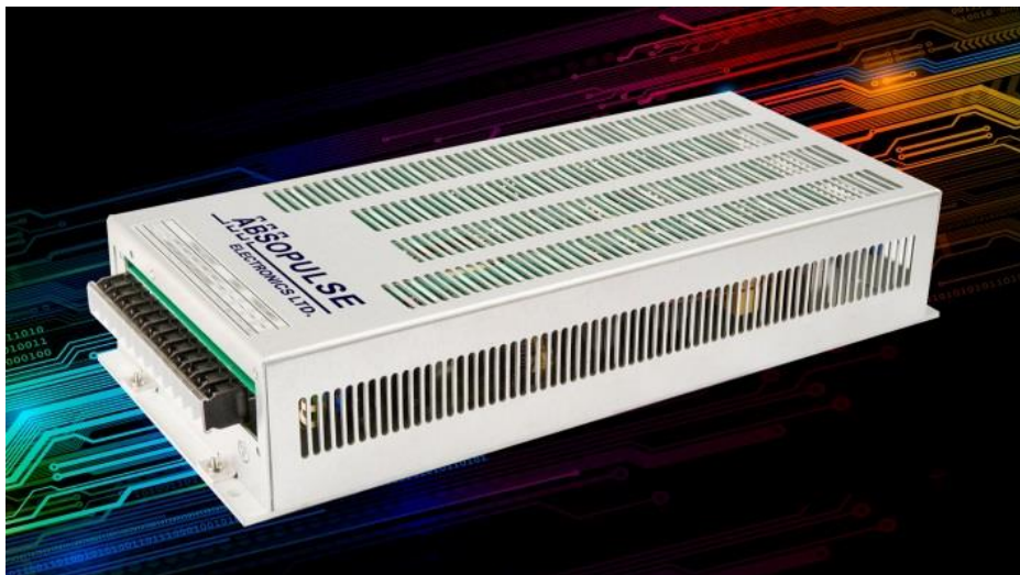
Figure. The HVI 500-1K-XX-FX series dc-dc converters accept a nominal input voltage of 1000 V with an 800-V to 1200-V operating input range. The 500-W units provide 36-V, 48-V, 110-V, 125-V or custom outputs.
