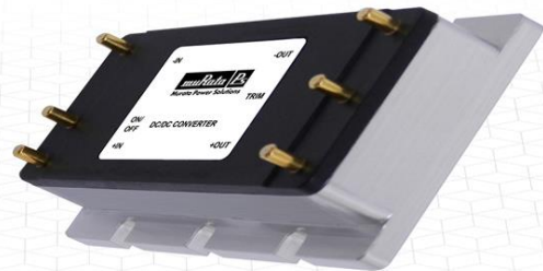
Murata IRQ series dc-dc converters output 5, 12, or 24 V at 100 W. They have a 3:1 wide input range of 57.6 to 160 V.
