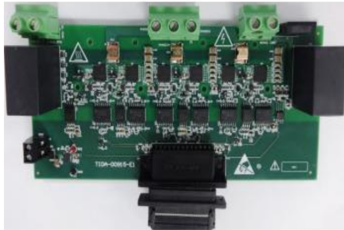
Fig. 1. TI's three-phase, gallium nitride-based inverter reference design helps engineers build 200-V, 2-kW ac servo motor drives and next-generation industrial robotics. The design is based on the company's LMG3410 600-V, 12-A GaN power module.
