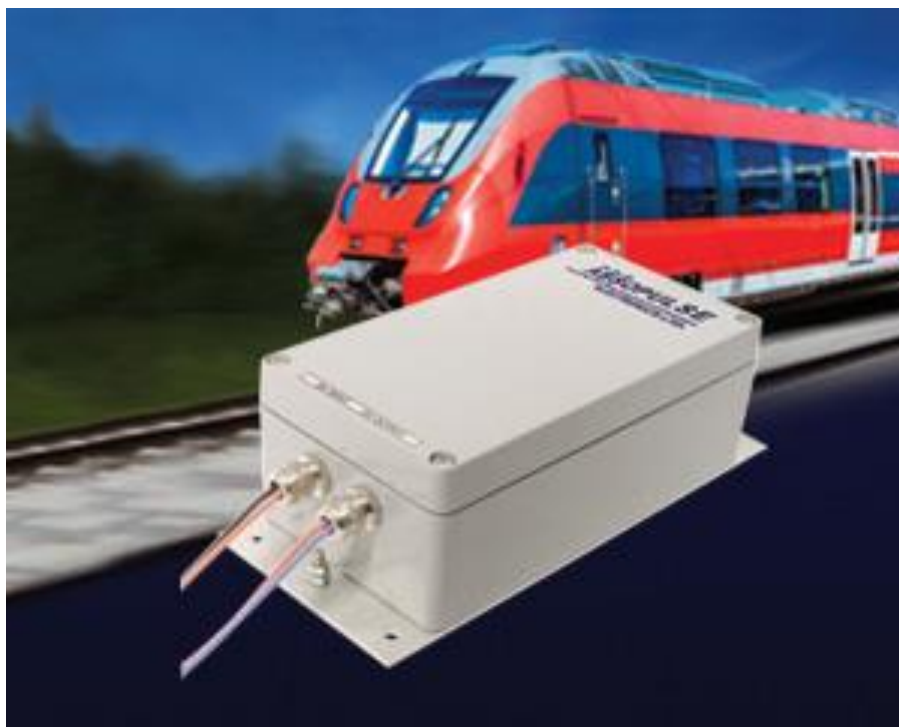
Figure. Installed in IP66-rated waterproof, die cast aluminum packages with sealed connectors, the RSI 30-D1 railway quality sinewave inverters are protected from the ingress of rain, humidity, sand, dust, metallic dust, oil and other contaminants. These inverters meet the requirements of EN50155 for electronic equipment used on railway rolling stock, comply with EN50121-3-2 (with heavy filtering) and also meet EN61000-4-2, EN61000-4-3, EN61000-4-4, EN61000-4-6 and related railway standards.
