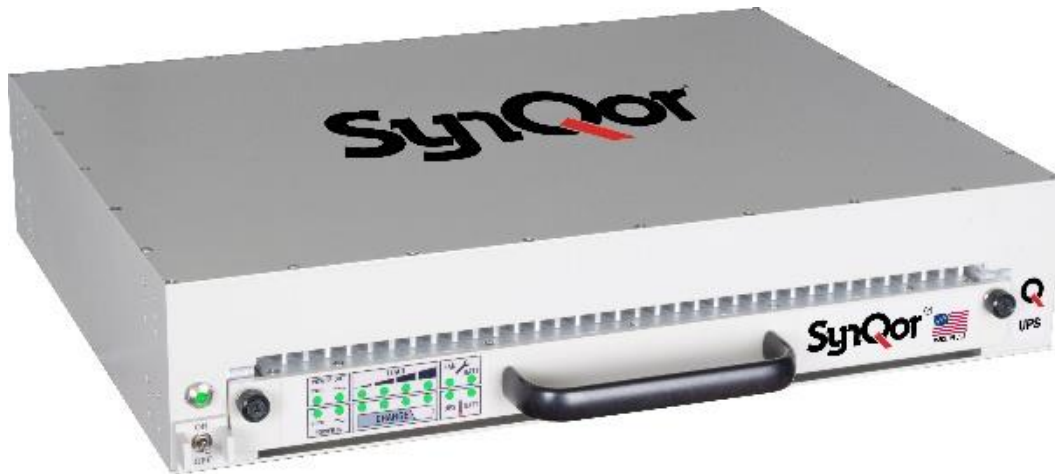
Figure. The UPS-1500-S-2S Shallow Depth Military-Grade UPS delivers 1250 W (1500 VA) of output power in a 2U high unit that is 17 in. wide x 13.6 in deep. The UPS specifies >10 minutes run-time at full power.
