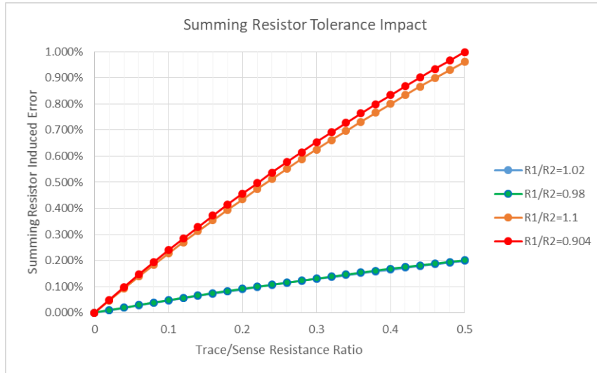
Fig. 7. Impact of summing resistor tolerance on the added current monitoring error.
