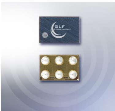
Fig. 1. Intended for use in portable devices, the GLF76321 IQSmart load switch draws just 7 nA in standby, which is negligible compared to the typical self-discharge of Li-ion batteries. This chip-scale packaged IC (shown on left) enables wearables, mobile and IoT devices to be shipped and stored with charged batteries so they can operate right out of the box. The GLF76321 includes integrated 1-ms slew rate control and output discharge functions.
