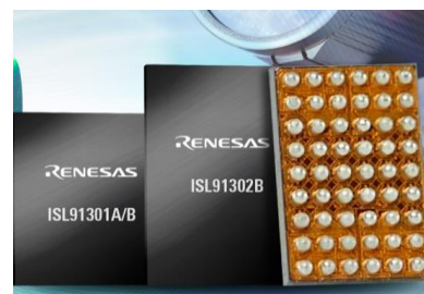
Fig. 1. The ISL91302B delivers up to 20 A and 94% peak efficiency in a 70-mm 2 solution size for application processors, AI processors, industrial MPUs, and FPGAs. This model is available in a dual-phase (2 + 2) configuration supporting 10 A from each output, a triple-phase (3 + 1) configuration supporting 15 A from one output and 5 A from the second output and a quad-phase (4 + 0) configuration supporting 20 A from one output. The ISL91302B's 2.551-mm x 3.670-mm, 54-ball WLCSP package is pictured on the right.
