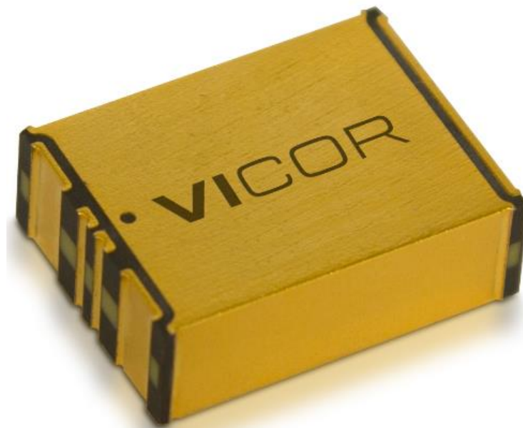
Figure. The 2317 NBM is a bidirectional converter capable of providing up to 750 W continuously at 48 V from 12 V, or at 12 V from 48 V, with over 98% peak efficiency in a 23-mm x 17-mm x 7-mm surface-mount package.
