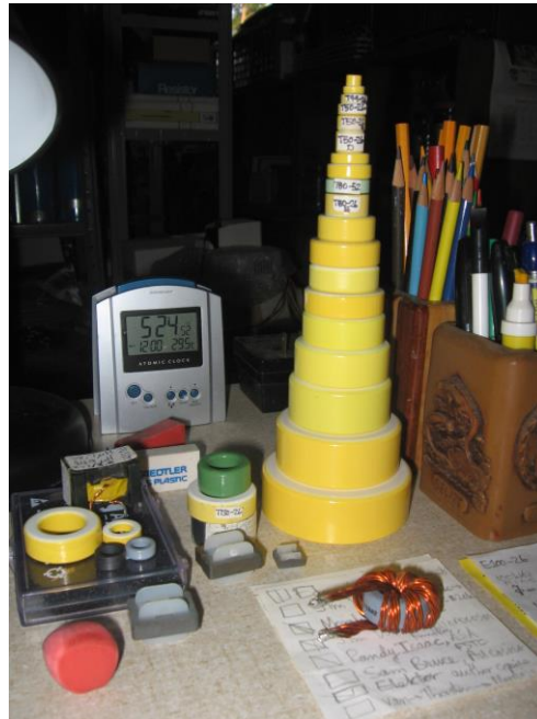
Fig. 4. Samples of (mostly) powdered-iron toroid cores. How can they be mounted on a circuit-board?
