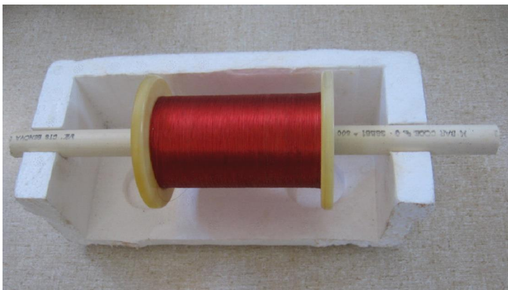
Fig. 1. Quick and easy spool holder, cut from the corner of styrofoam packaging with ½-inch PVC pipe section.
