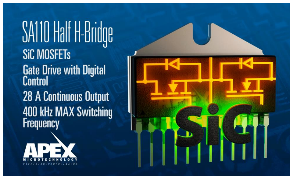
Fig. 1. The SA110 is introduced as the first high-current, high-voltage half H-bridge to combine SiC MOSFETs with gate drive in a single module. Integrating the gate drive improves switching behavior as parasitics are reduced and easier to control.
